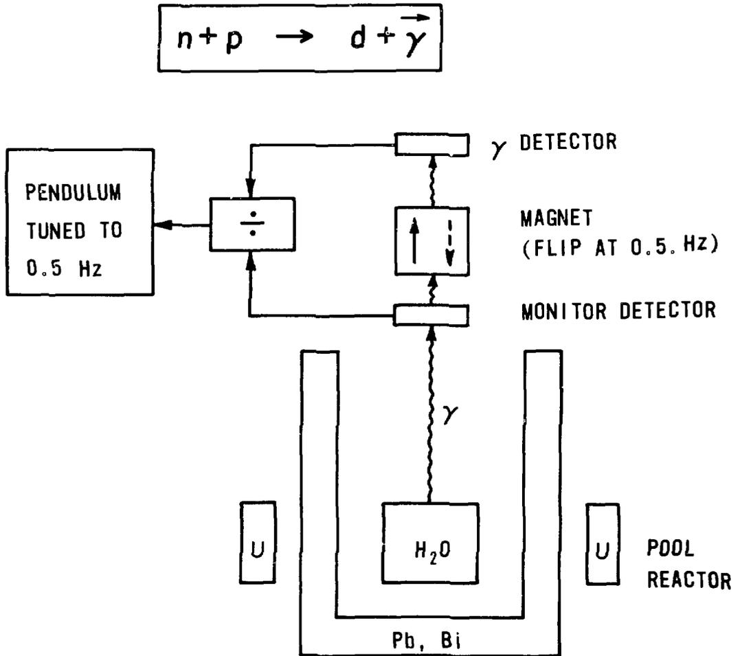
Figure 3 Schematic illustration of the  $n + p \rightarrow d + \vec{\gamma}$  experiment of ref. 14.
