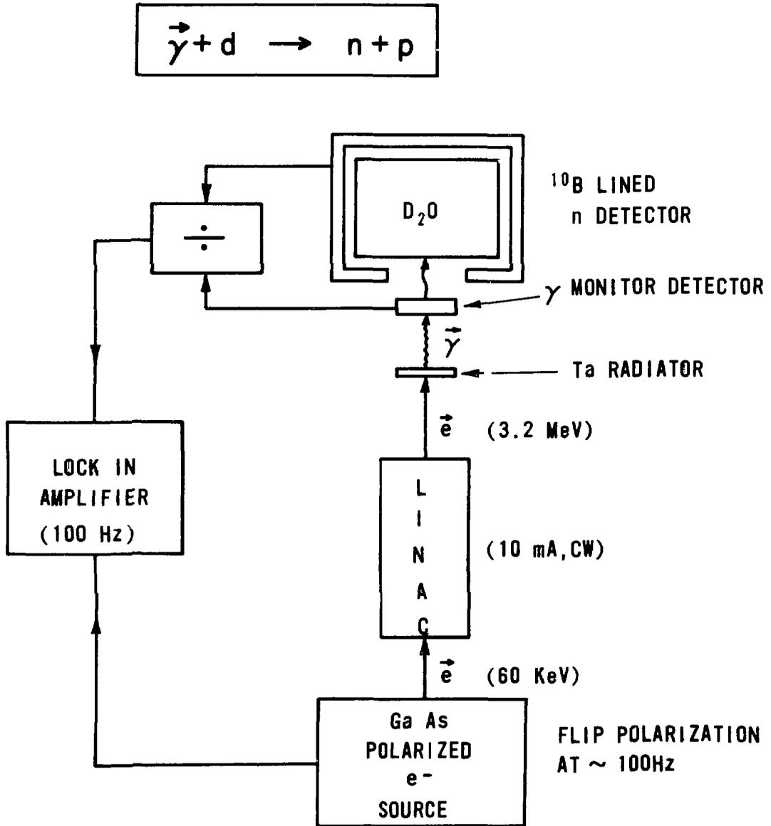
Figure 4 Schematic illustration of the  $d + \vec{\gamma} \rightarrow n + p$  experiment in preparation at Chalk River.
