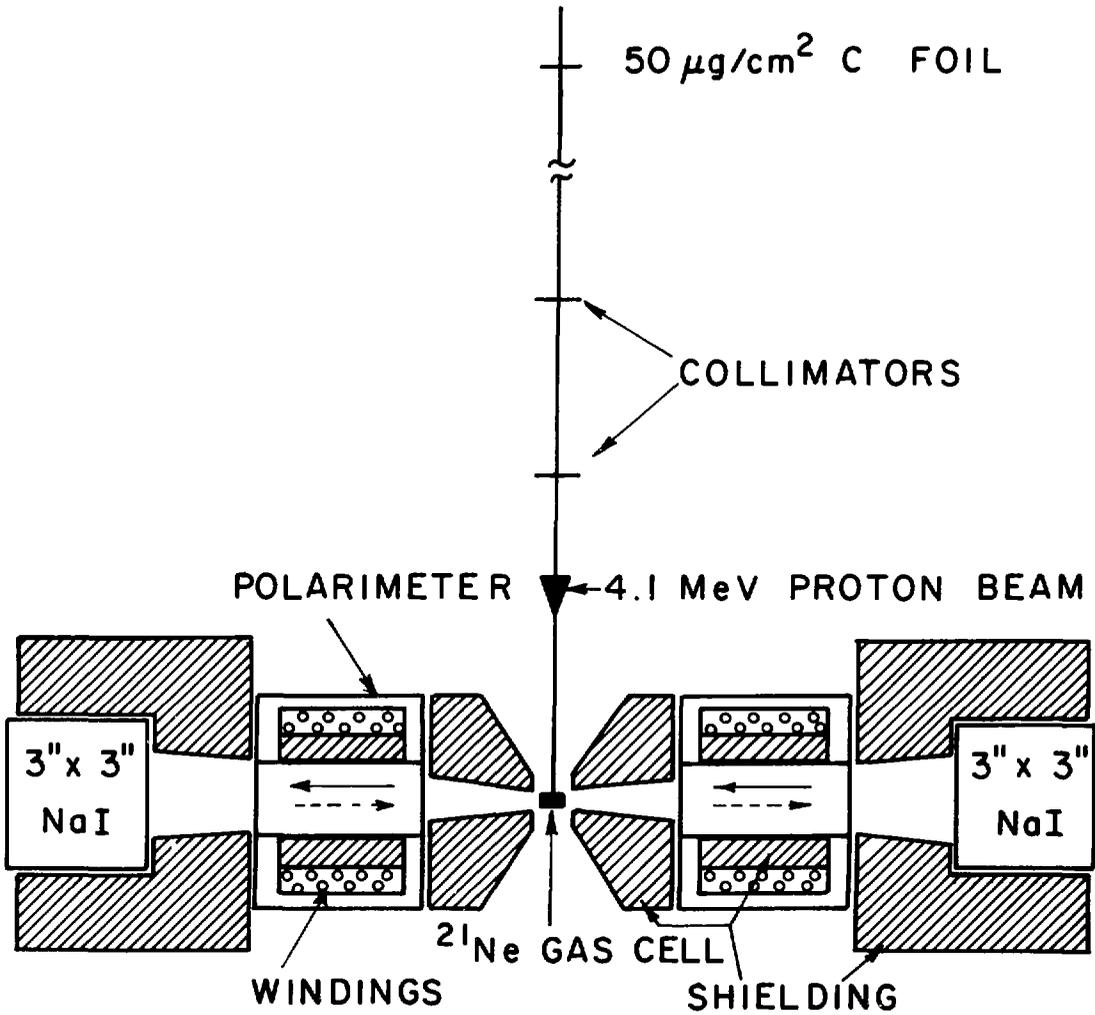
Figure 6 Schematic diagram of the apparatus used in the measurement of parity mixing in  $^{21}\text{Ne}$ . The  $50 \mu\text{g}/\text{cm}^2$  carbon foil was used to diffuse the beam and prolong the lifetime of the molybdenum foil on the  $^{21}\text{Ne}$  gas cell.
