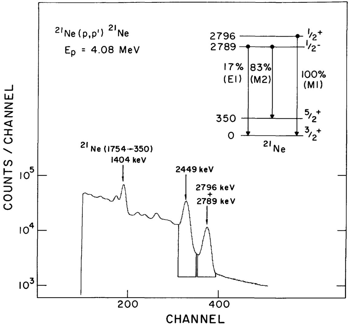
Figure 7 Spectrum of gamma rays from the  $^{21}\text{Ne}(p,p')^{21}\text{Ne}$  reaction obtained from one of the NaI(Tl) detectors mounted behind the polarimeter. Windows used to determine total counts in the 2.4 and 2.9 MeV photopeaks are indicated.
