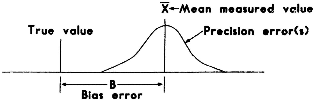
Figure 4. Measurement error.
