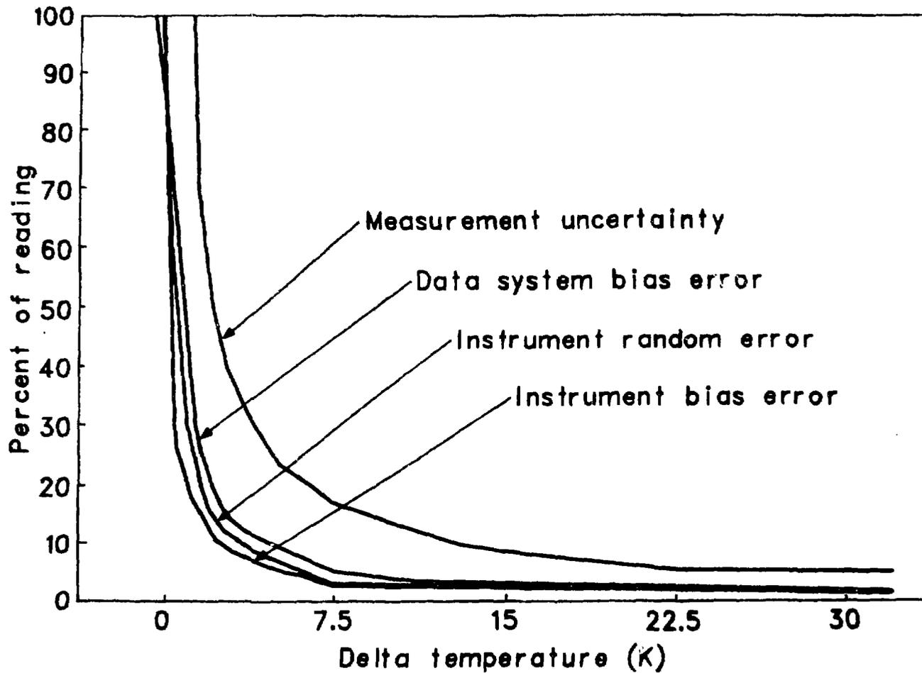
Figure 3. Test dependent uncertainty for Type T (copper-constantan) differential thermocouple measurement.
