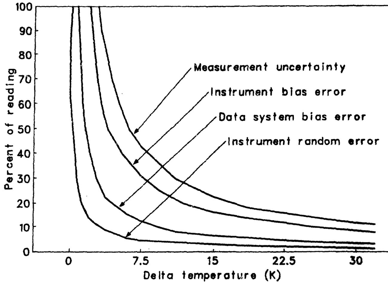
Figure 2. Test independent uncertainty for Type I (copper-constantan) differential thermocouple measurement.
