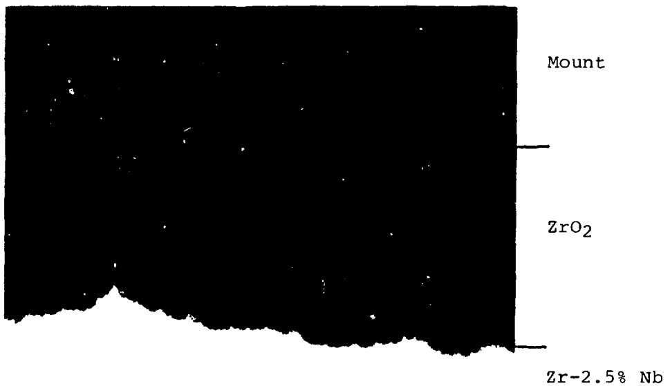
b. Thick compact oxide on specimen end (x1000)
