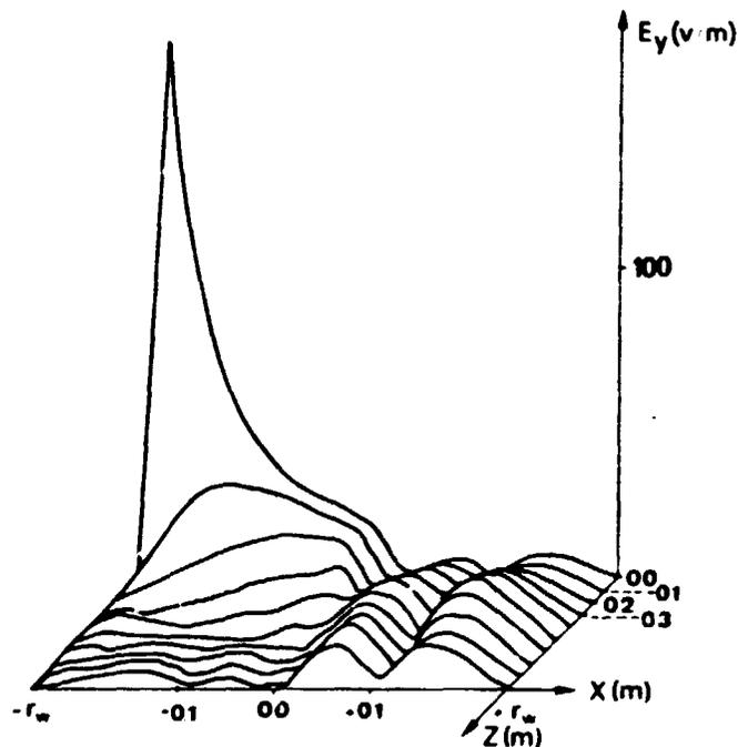
FIG. 3 : Electric field distribution. Inverse Fourier spectrum of fig. 2.
