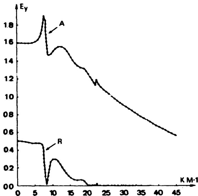
FIG. 2 : Fourier spectrum of the electric field at  $X = R_1$ . Antenna on the high field side.
