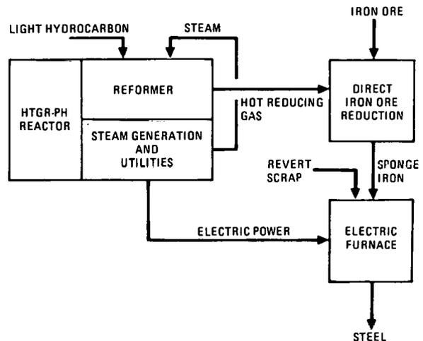
Figure 4 HTGR for direct reduction of iron ore
