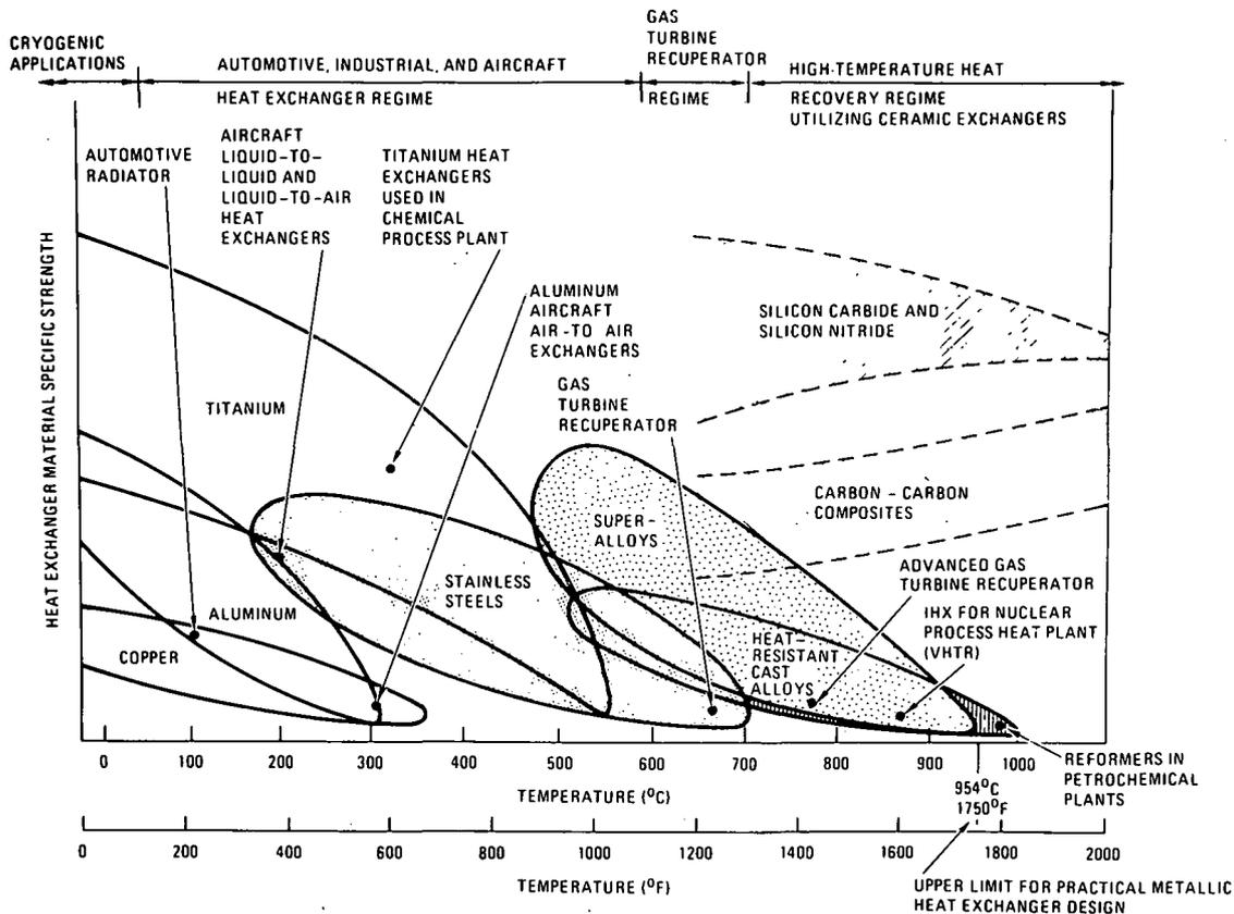
Figure 6 Approximate operating boundaries for various heat exchanger materials
