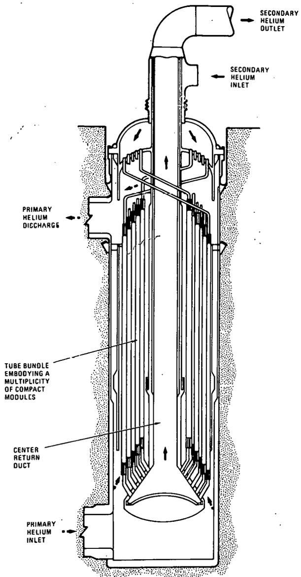
Figure 5 Overall view of modular, straight-tube IHX concept for HTGR-PH plant
