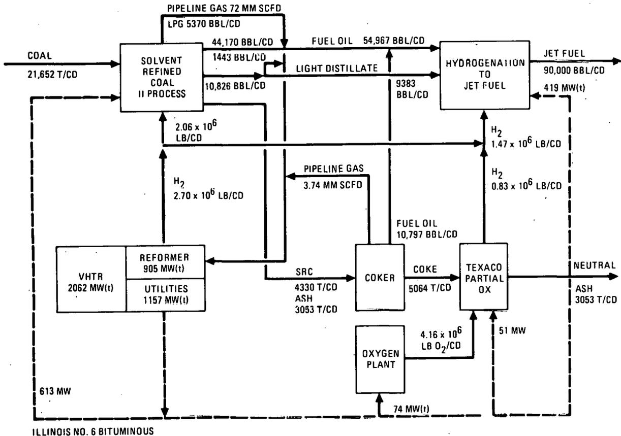
Figure 3 Coal to jet fuel, using VHTR reforming for H<sub>2</sub> (prime) utilities
