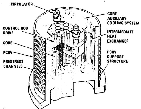
Figure 1 Nuclear heat source arrangement for 842-MW(t) HTGR-PH plant
