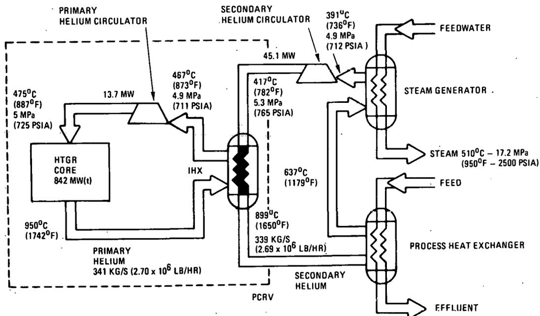
Figure 2 Cycle diagram for 950°C HTGR-PH plant
