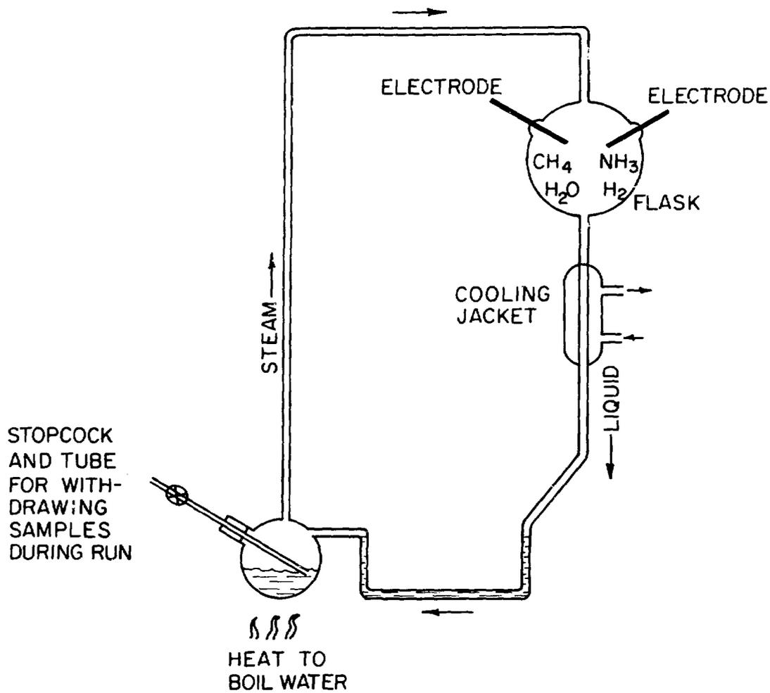
Fig.2. Representation of the Miller-Urey discharge apparatus. Organic compounds which form collect in the condensed water in the lower flask.
