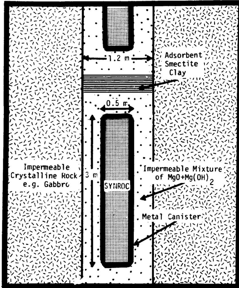
Fig. 4. Disposal of high-level waste (immobilized in SYNROC) within a hole drilled in impermeable crystalline rock eg. gabbro. Canisters are mechanically supported and fully sealed within the hole by an impermeable, pore-free mantle consisting of a mixture of periclase (MgO) and brucite (Mg(OH)<sub>2</sub>). Each unit is separated by a further barrier consisting of impermeable and adsorbent clay.
