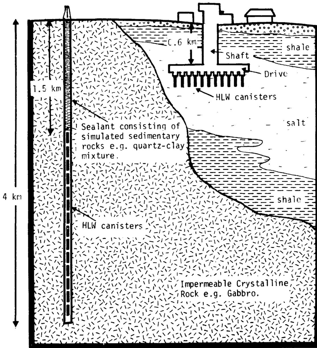
Fig. 5. Notional comparison of drill hole disposal concept with mined geologic repository.
