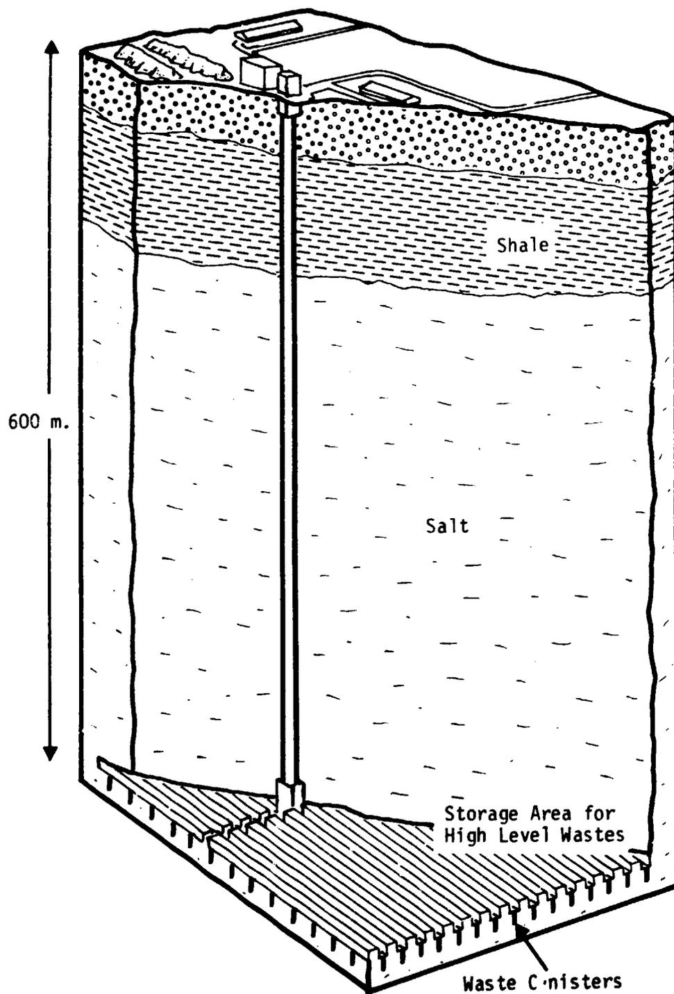
Fig. 3. Design for large mined repository in salt (after Cohen, 1977).
