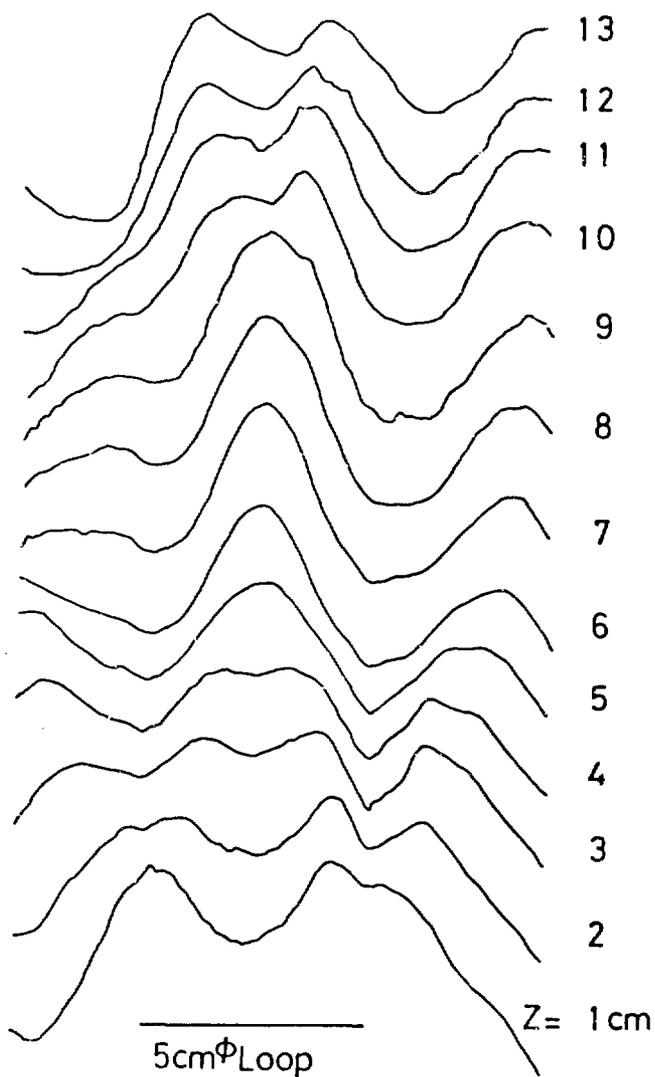
Fig. 13. Resonance cone fields radiated from a ring source with a large oscillating amplitude.
