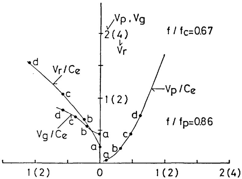
Fig. 6. Theoretical ray velocity ( $V_r$ ), group velocity ( $V_g$ ), and phase velocity ( $V_p$ ) surfaces of the thermal mode (the oblique electron mode).  $C_e$ : the electron thermal velocity.
