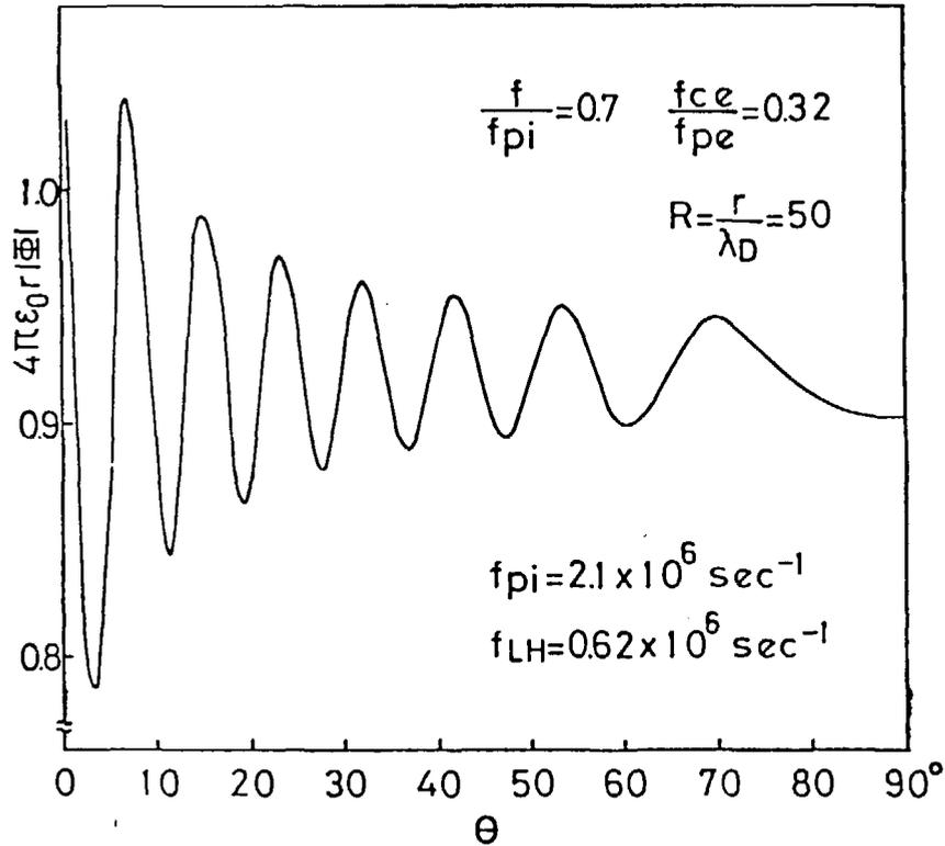
Fig.17. Potential amplitude radiated from a point source near the lower hybrid frequency, i. e. an interference pattern between lower hybrid and ion acoustic waves.
