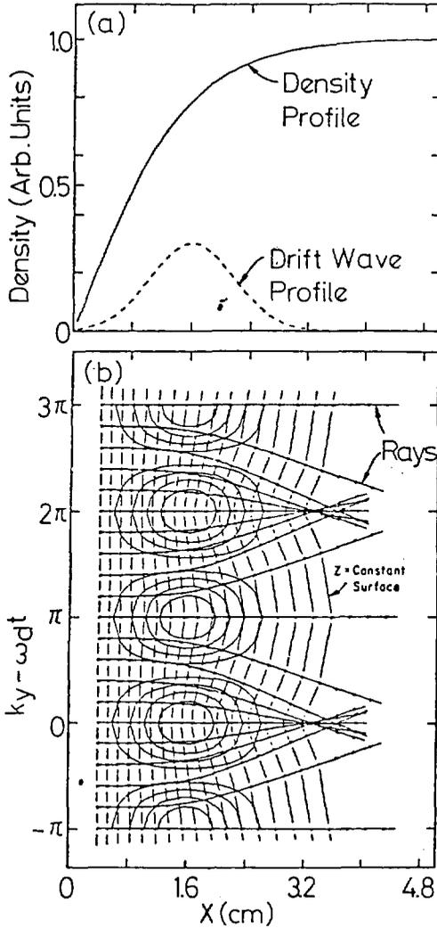
Fig.18. (a) Density and drift-wave profiles (b) Ray refraction of resonance cone fields due to drift waves. Concentric ellipses are constant drift-wave amplitude contours (Ref.33).
