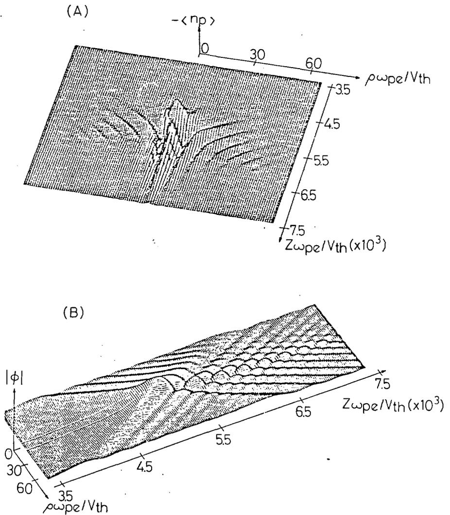
Fig. 27. Magnitude of the complex potential radiated from a ring source, displaying the interference structure due to thermal effects.  $f/f_{pe} = 0.02$ ,  $\rho_o \omega_{pe}/v_{th} = 270$  (B), the first-order density depression due to the ponderomotive force for  $f/f_{pe} = 0.02$  (A) (Ref. 62)
