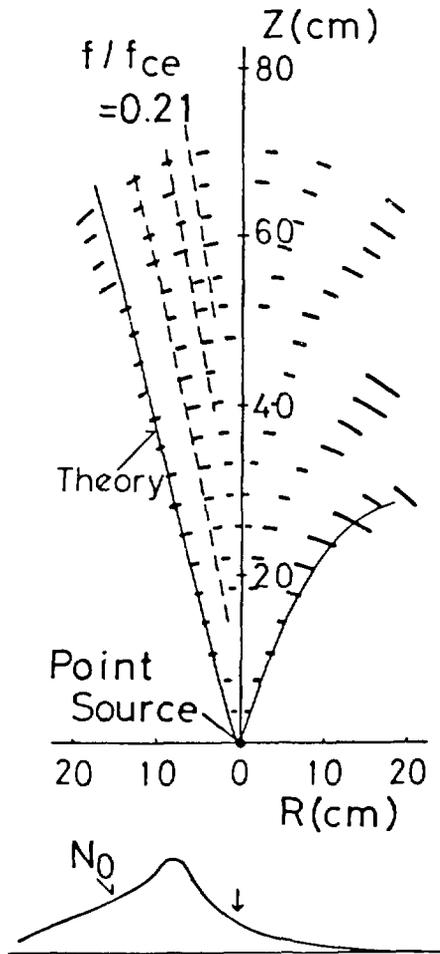
Fig. 5. Trajectories of resonance cones (a) and thermal modes (b) in an inhomogeneous plasma. Solid lines are the theoretical resonance cone trajectories. Dashed lines are theoretical wave fronts obtained from ray velocity surface of oblique electron mode.  $f_{pe}/f_{ce} \approx 1$  at the point source.
