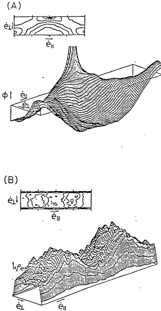
Fig. 29. Numerical electrostatic potential associated with lower hybrid resonance cone excited point source,  $f/f_{pe} = 0.35$ ,  $f_{ce}/f_{pe} = 1$  (A), Typical density profile at peak density depression averaged over one oscillation period (B), (Ref.101).
