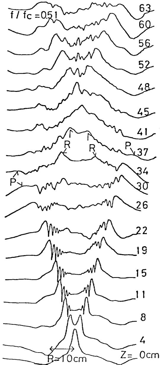
Fig. 11. Ducted resonance cone fields and thermal modes in an inhomogeneous magnetoplasma column. "R" and "P" are reflected and refracted cone fields at the electron plasma frequency layer.
