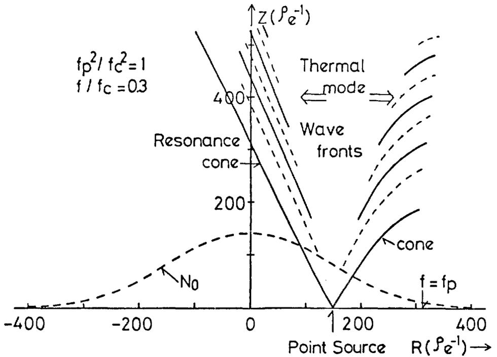
Fig. 25. Theoretical resonance cone fields and wave fronts of thermal modes radiated from a point source in an inhomogeneous plasma, which are derived from a kinetic theory (Ref. 59).
