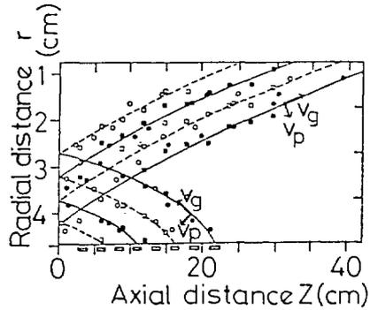
Fig. 16. Lower hybrid waves launched by the modified Millman circuit. Experimental plots for the contours of constant phase, where ●, ■ are for peaks and ○, □ for troughs (Ref. 30).
