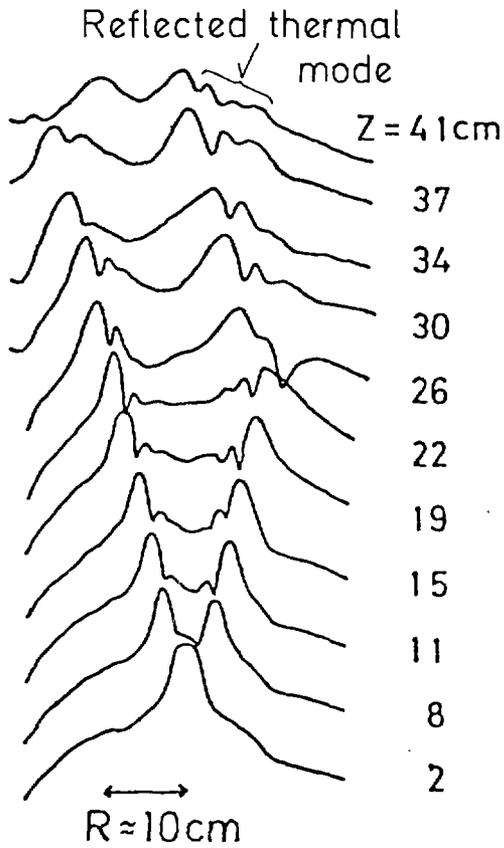
Fig. 9. Reflected thermal modes from the layer near the electron plasma frequency in an inhomogeneous magnetoplasma column.
