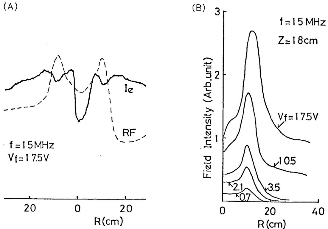
Fig. 31. (A) Resonance cone fields radiated from a point source when an applied power is varied. (B) Electron density profile and the corresponding amplitude of resonance cone rf fields under an application of high power fields.
