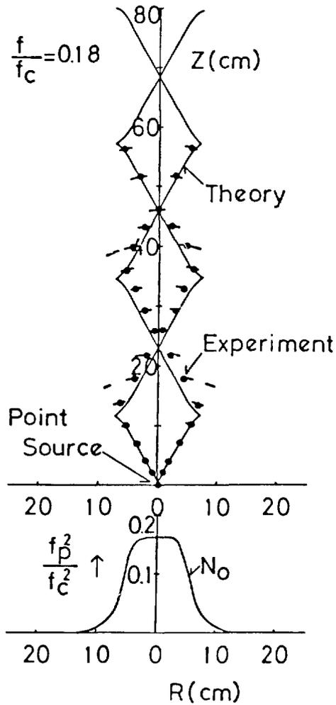
Fig. 3. Experimental and theoretical trajectories of resonance cone fields radiated from a point source in a magnetized plasma column where reflections occur at the electron plasma frequency layer. Bottom figure is the corresponding density profile.
