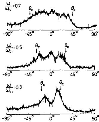
Fig. 23. Typical patterns of low frequency resonance cone fields near the ion cyclotron frequency. " $\theta_c$ " indicates the angle of low frequency resonance cone.
