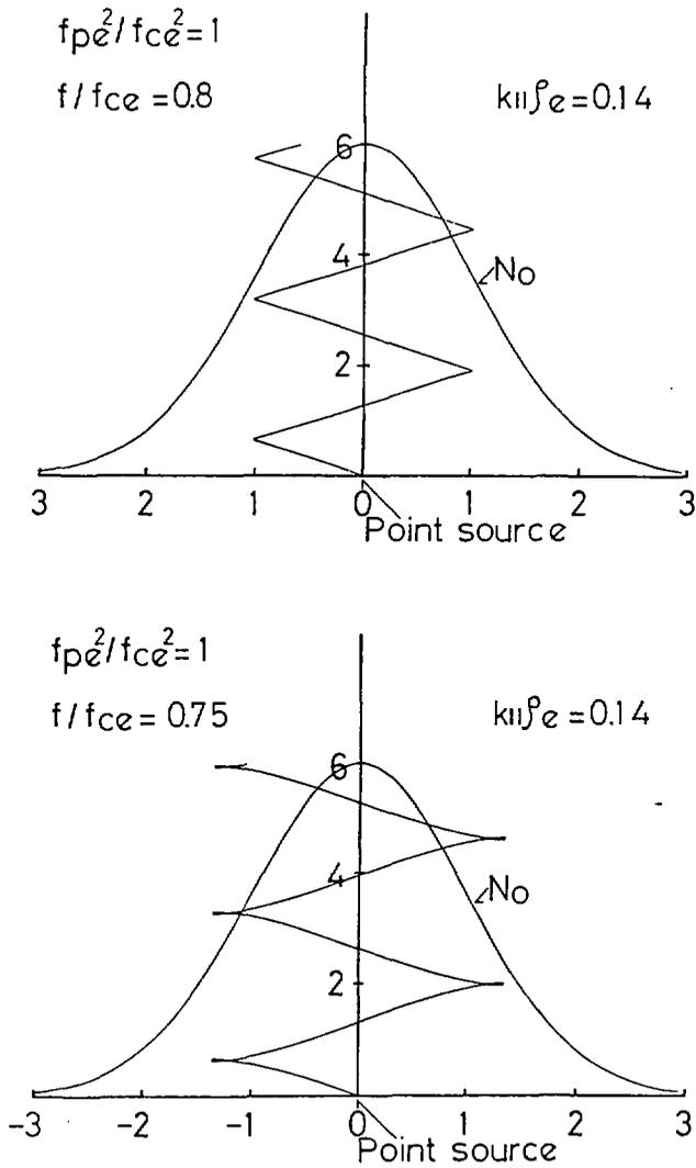
Fig. 24. Theoretical ray trajectories of localized rf fields in an inhomogeneous magnetoplasma column, in which thermal effects are included (Ref. 56).
