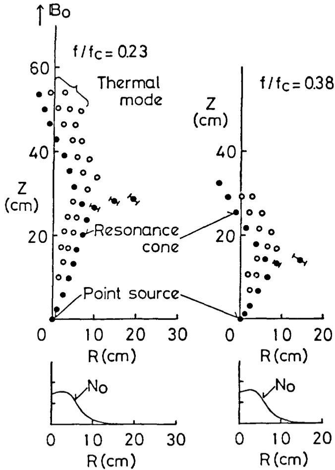
Fig.10. Reflection of thermal modes associated with reflection and refraction of resonance cone fields in an inhomogeneous plasma. The electron plasma frequency layer is at the point where the cone fields are reflected and refracted.
