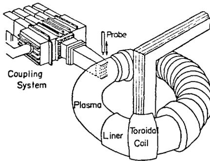
Fig. 21. Schematics of a waveguide coupling system of the JFT-2 tokamak for lower hybrid heating (Ref. 43)
