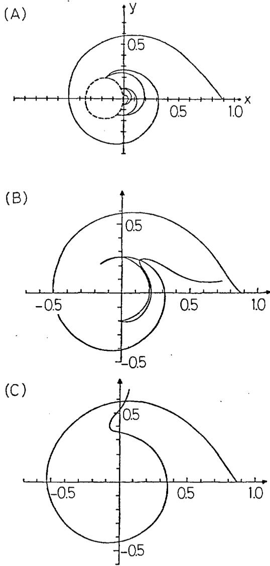
Fig. 30. Ray trajectories in  $r$ - $\theta$  plane in toroidal plasmas. The ray makes successive bounces off the lower hybrid surface (A). Thermal effects come into play after the first few bounces, and the wave mode-converted to a hot plasma wave (B:  $T_e = T_i = 100\text{eV}$ , C:  $T_e = T_i = 1\text{keV}$ ), (Ref. 114).
