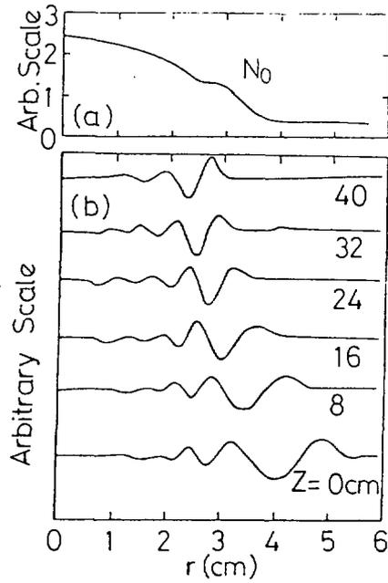
Fig. 15. Interferometer signal of radial lower hybrid wave field for a sequence of axial positions (b) and density profile (a). He gas.  $B=1.3\text{kG}$ ,  $f=20\text{MHz}$ . (Ref. 26)
