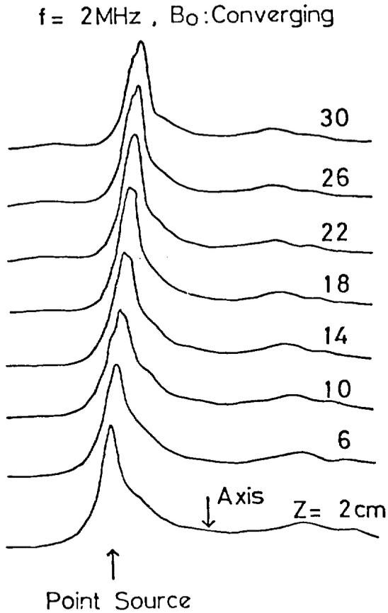
Fig.19. (A) Lower hybrid cone radiated from a point source in a converging magnetic field. (B) Resonance cone fields radiated from a point source in a converging magnetic field. Point source is located at  $Z=0\text{cm}$ . The axis means the magnetic axis of the converging field.
