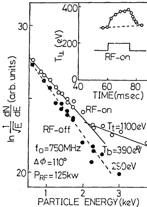
Fig. 22. Increase of ion temperature and a change of ion distribution function during lower hybrid rf heating in JFT-2 tokamak (Ref. 41)
