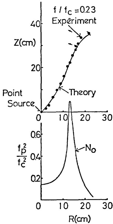
Fig. 2. Experimental and theoretical resonance cone trajectory in an inhomogeneous magnetoplasma. Bottom figure is the density profile.
