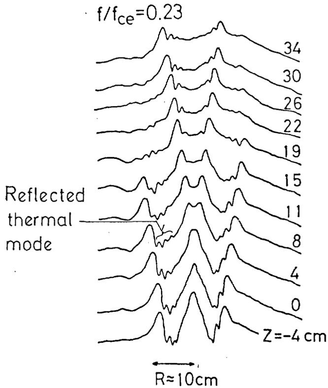
Fig. 8. Reflected thermal modes from an insulator disk which is placed perpendicular to magnetic field at  $Z = -20$  cm.
