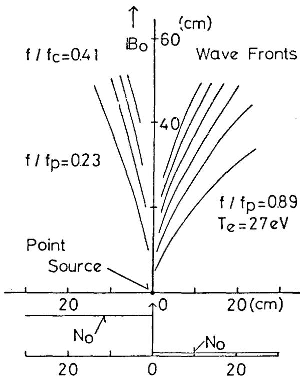
Fig. 7. Theoretical wave fronts of the thermal mode which are obtained from such a ray velocity surface as Fig. 6. Two cases of plasma density are indicated.
