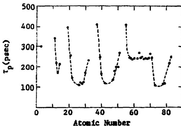
Fig. 1 - Variation of the mean positron lifetime with atomic number in the well annealed bulk lattice (8).
