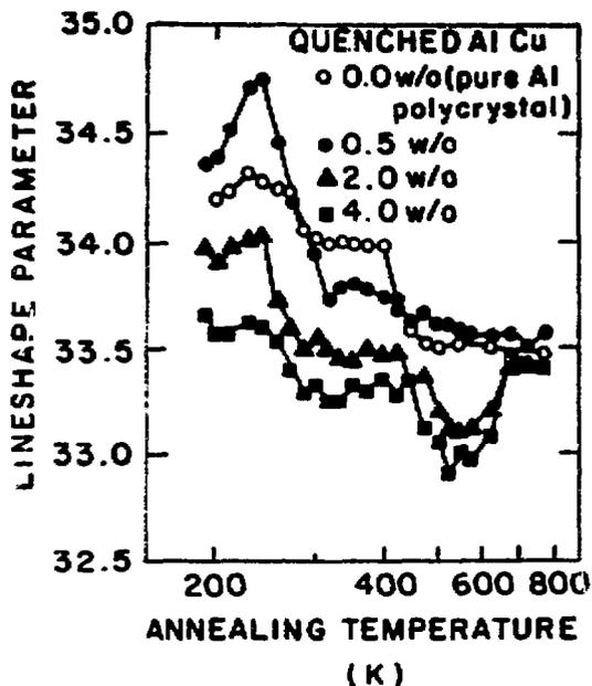
Fig. 13 - Doppler-broadening lineshape parameter S (x100) as a function of isochronal annealing temperature (log scale) (65).
