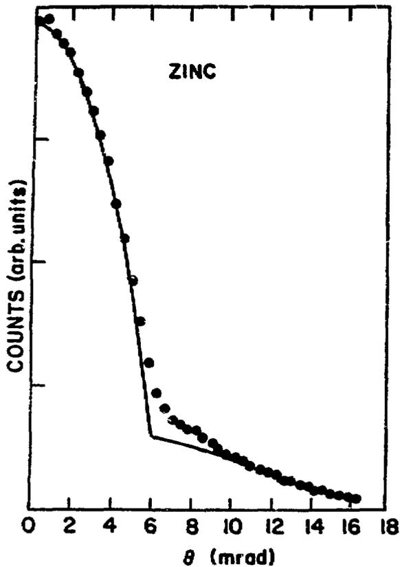
Fig. 3 - Angular correlation distribution for polycrystalline Zn [(12) and references therein].
