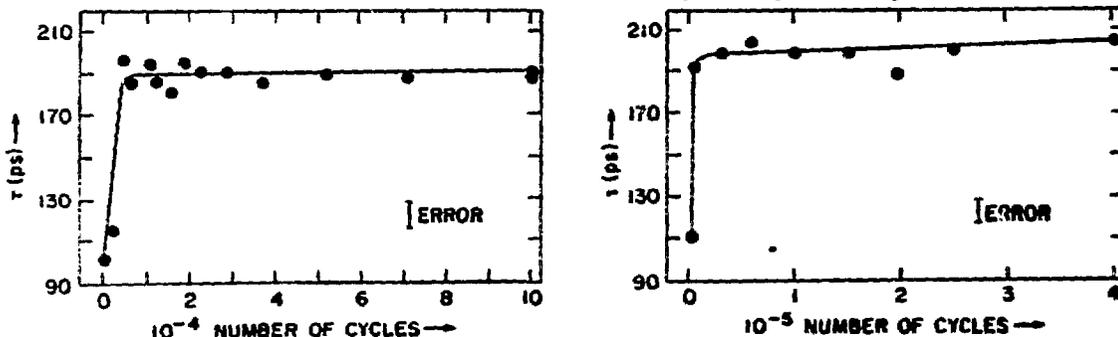
Fig. 11 - (a) The mean positron lifetime in pure Ni as a function of cyclic deformation. (b) in Ni - 66.5% Co (61).
