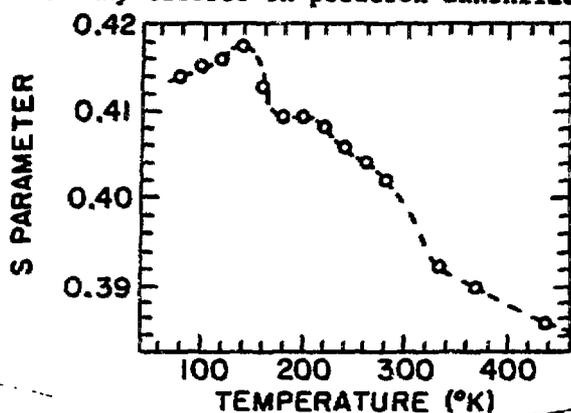
Fig. 6 - Doppler-broadening S parameter as a function of isochronal annealing temperature for Zn single crystals after deformation (10%) at 77K. All data points were taken at a sample temperature of 77K.
