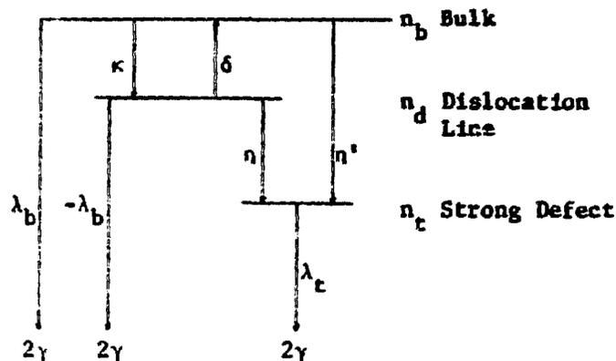
Fig. 10 - Schematic representation of the trapping model (53).  $\kappa$ ,  $\eta$ , and  $\eta'$  are trapping rates to the states shown.  $\delta$  is the detrapping rate from dislocations.  $\lambda_b$  and  $\lambda_c$  are annihilation rates.
