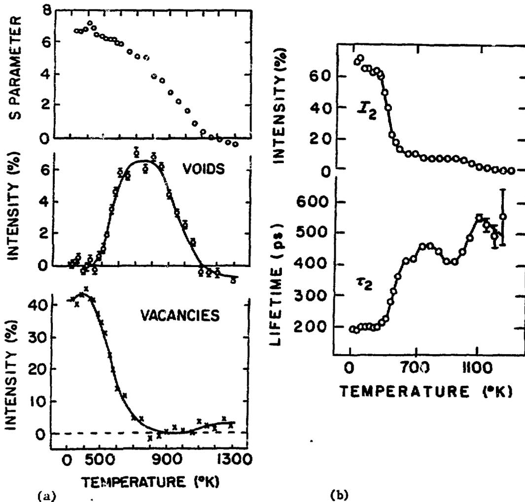
Fig. 8 - Results of isochronal annealing studies of electron irradiated Mo. (Eldrup et al. (29)).
