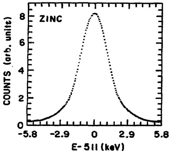
Fig. 2 - Doppler-broadening spectrum from a well annealed 99.999% Zn sample.
