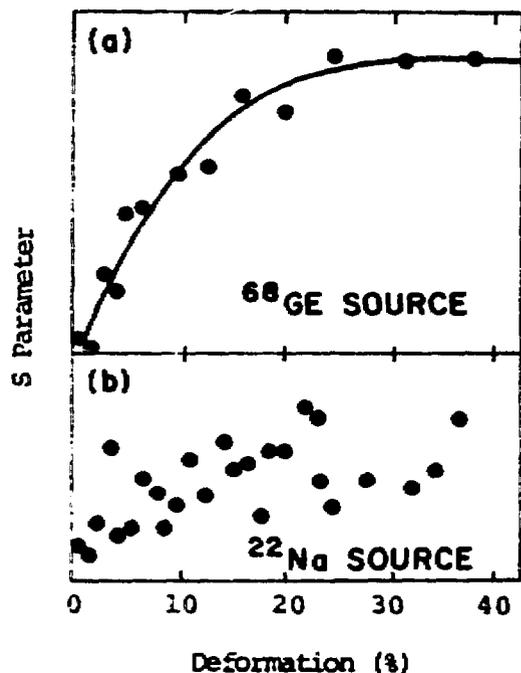
Fig. 14 - Variations of the Doppler-broadening annihilation line width with deformation in rolled Al clad 2024 samples irradiated with (a)  $^{68}\text{Ge}$  positrons (b)  $^{22}\text{Na}$  positrons (J. Eady et al. unpublished).
