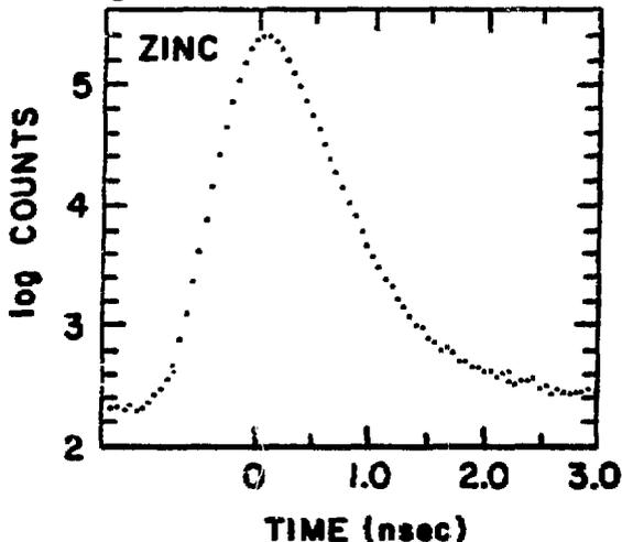
Fig. 4 - Positron lifetime spectra for well annealed 99.999% zinc single crystal
