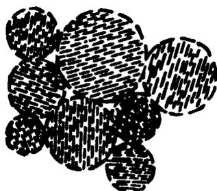
Fig. 3. Schematic microstructure of compacted "air-dry" MX-80.
