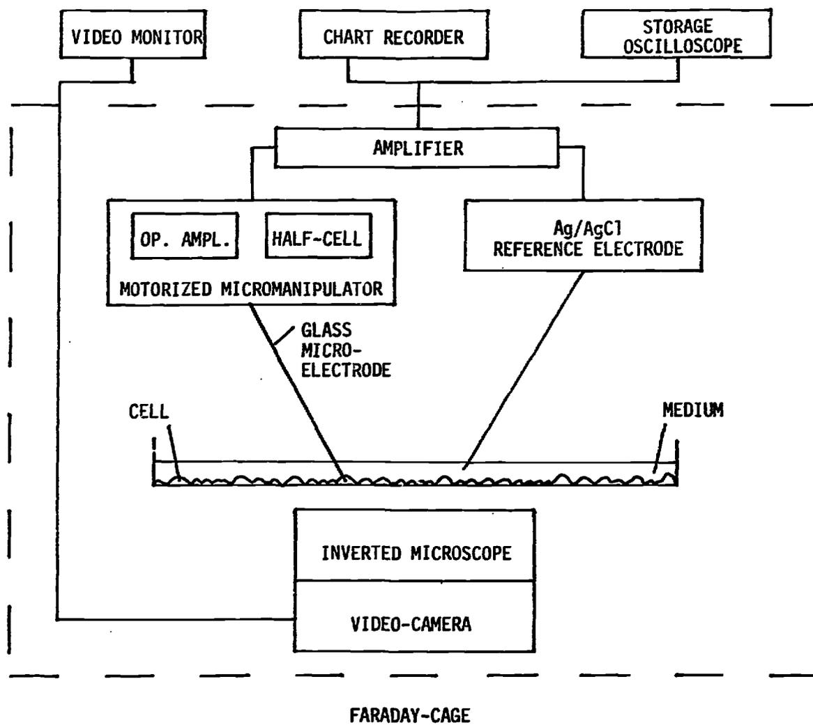
Fig. 1 EXPERIMENTAL SET-UP USED FOR INTRACELLULAR ELECTRICAL MRP-RECORDINGS FROM HUMAN CELLS
