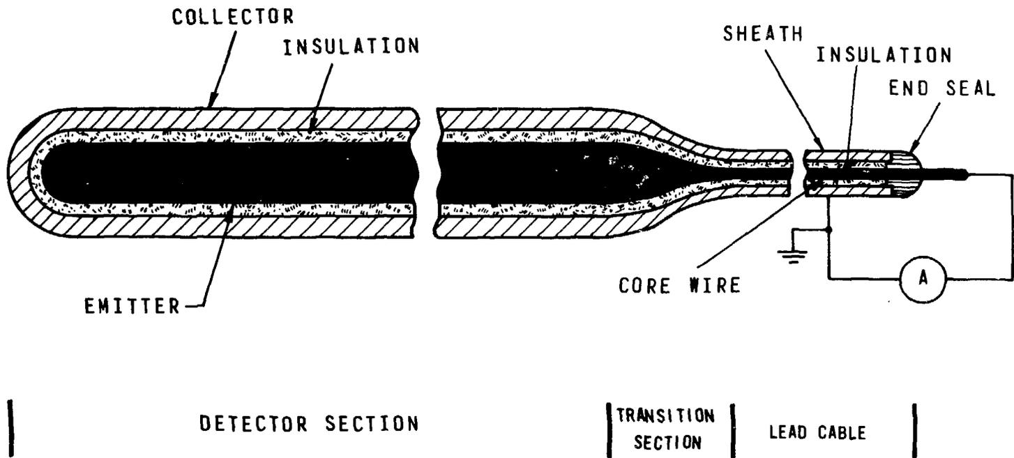
FIGURE 5 SCHEMATIC OF A SELF-POWERED FLUX DETECTOR
