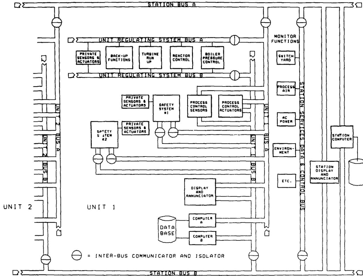
FIGURE 9 CONCEPTUAL BLOCK DIAGRAM OF A TOTAL INFORMATION NETWORK
