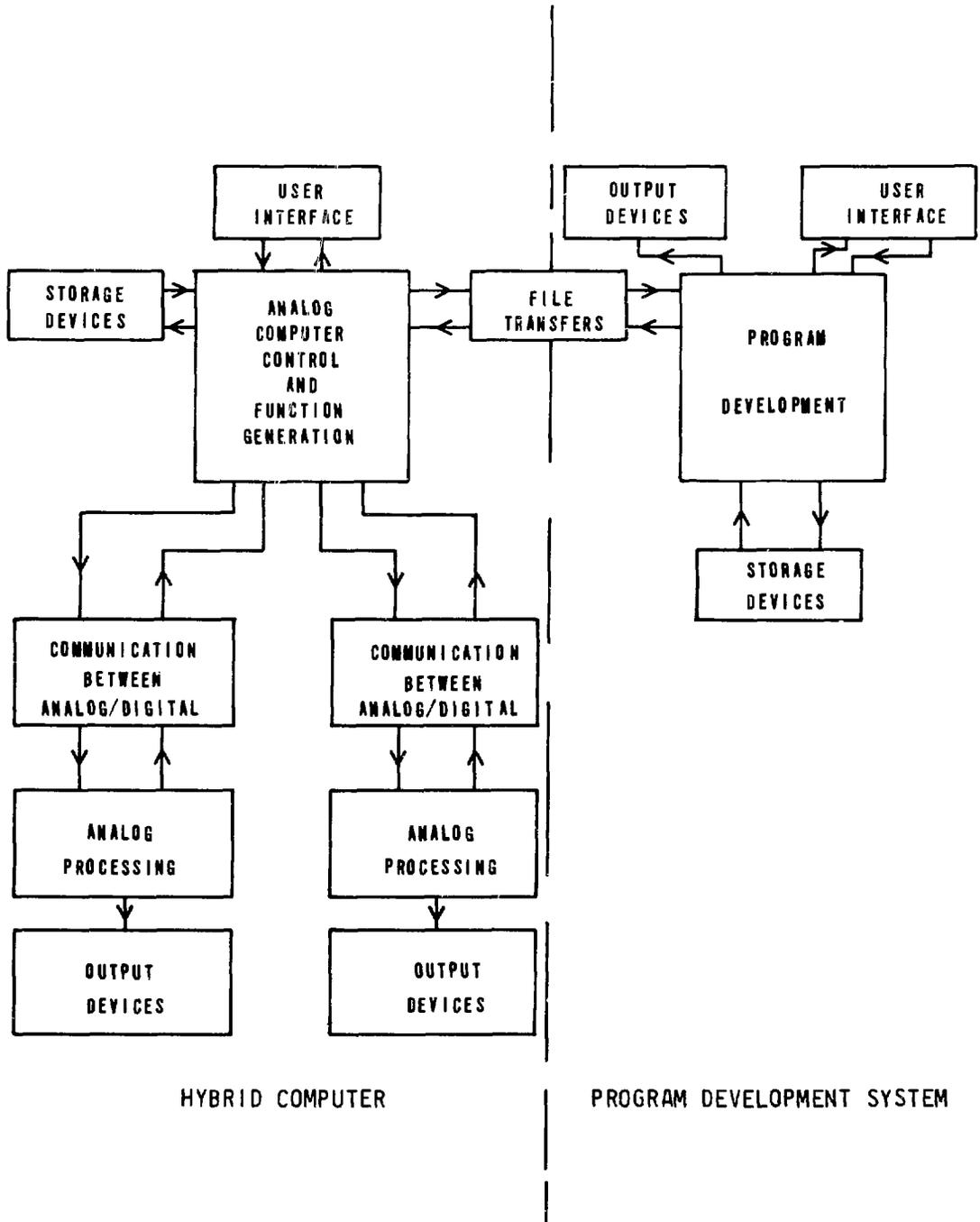
FIGURE 2 FUNCTIONAL DIAGRAM OF THE DYNAMIC ANALYSIS FACILITY
