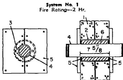
System number 1 is shown in Figure 3. The elements of this system are as follows: The wall (1) is nominally an 8 inch thick wall fabricated of concrete block, or common brick laid up with mortar. It must be a minimum 2
