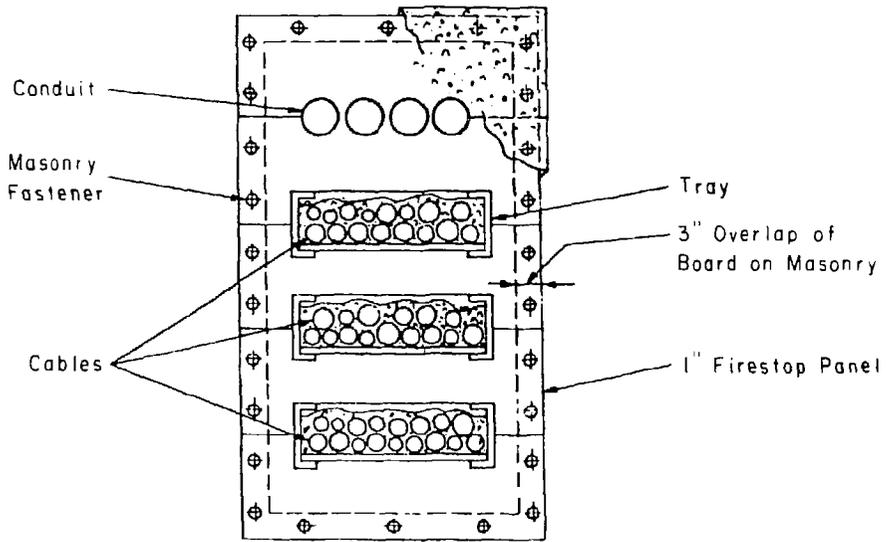
Fig. 15. Multiple Tray Penetration with Suggested Subdivision of Panels.
