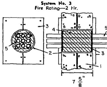
System number 3 is shown in Figure 5. The wall (1), forming materials (3) and fill, void, or cavity materials (4) are as described for system 1. The steel framing (2) is a nominal 6 inch diameter, 0.25 inch wall steel pipe rigidly attached to the wall. The cables (5) are an aluminum conductor, PVC jacket 4/C, No. 14 AWG. There is a maximum 40 percent cable fill.
