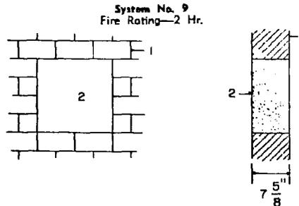
System number 9 is shown in Figure 11. The wall (1) and maximum opening size are as described for system 7. The fill, void, or cavity material (2) is as described for system 6.
