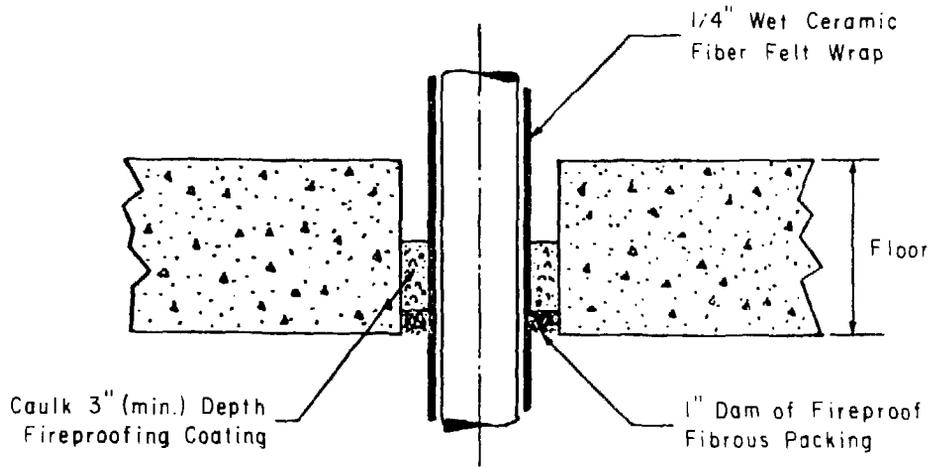
Fig. 16. Sealing Pipes or Ducts Through Wall or Floor Penetration.
