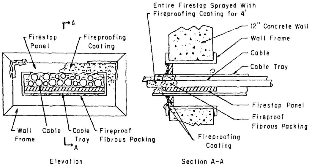
Fig. 12. Penetration Seal for Typical Prefabricated Channel Frame Wall Opening.
