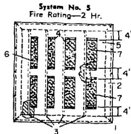
System number 5 is shown in Figure 7. The wall is as described above for system 1. The maximum size wall opening is 48 inches high and 48 inches wide. The steel framing (2) and the support angle (3) are as described above for system 2. The cable tray (4) is 18 inches wide, 4 inches high of solid, 16 gauge minimum galvanized steel. It is tack welded at each side to the channel supports. The forming materials (5) and fill, void, or cavity
