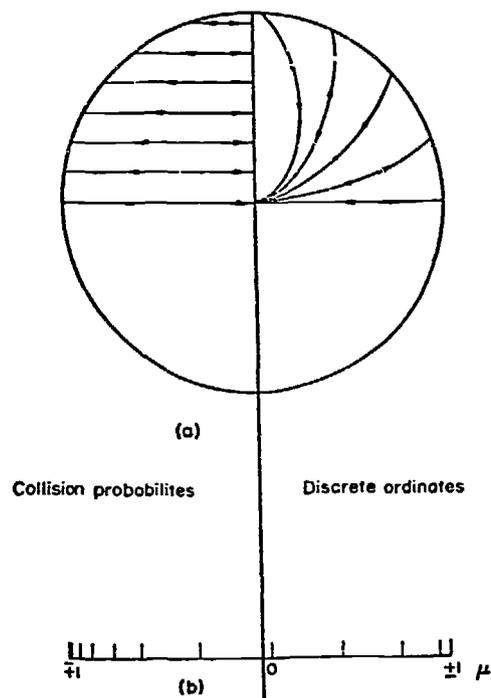
FIG. 8. (a) Typical tracking schemes for collision probabilities discrete ordinates. (b) Angular representations at outer surface. Collision probability and discrete ordinate tracking schemes in curved geometry.
