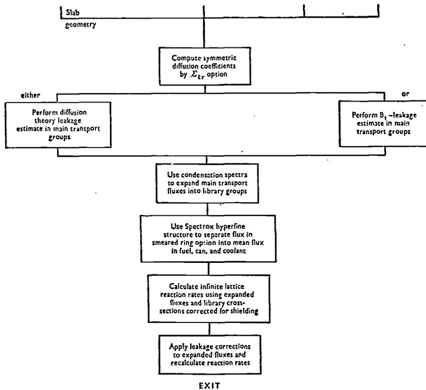
FIG. 1. Block diagram of computational sequences in WIMS
