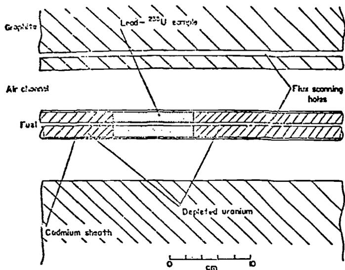
FIG. 5. Experimental Arrangement in Measuring Cell
