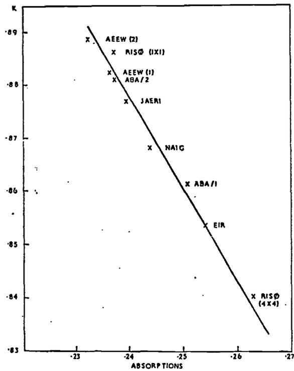
EIGENVALUE VS ABSORPTIONS IN POISON PIN
