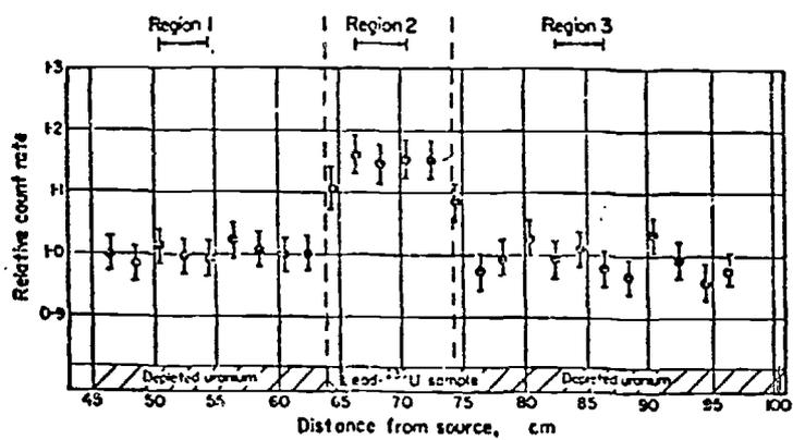
FIG. 6.  $^{235}\text{U}$  fission chamber scan with 10-cm lead/ $^{235}\text{U}$  sample.
