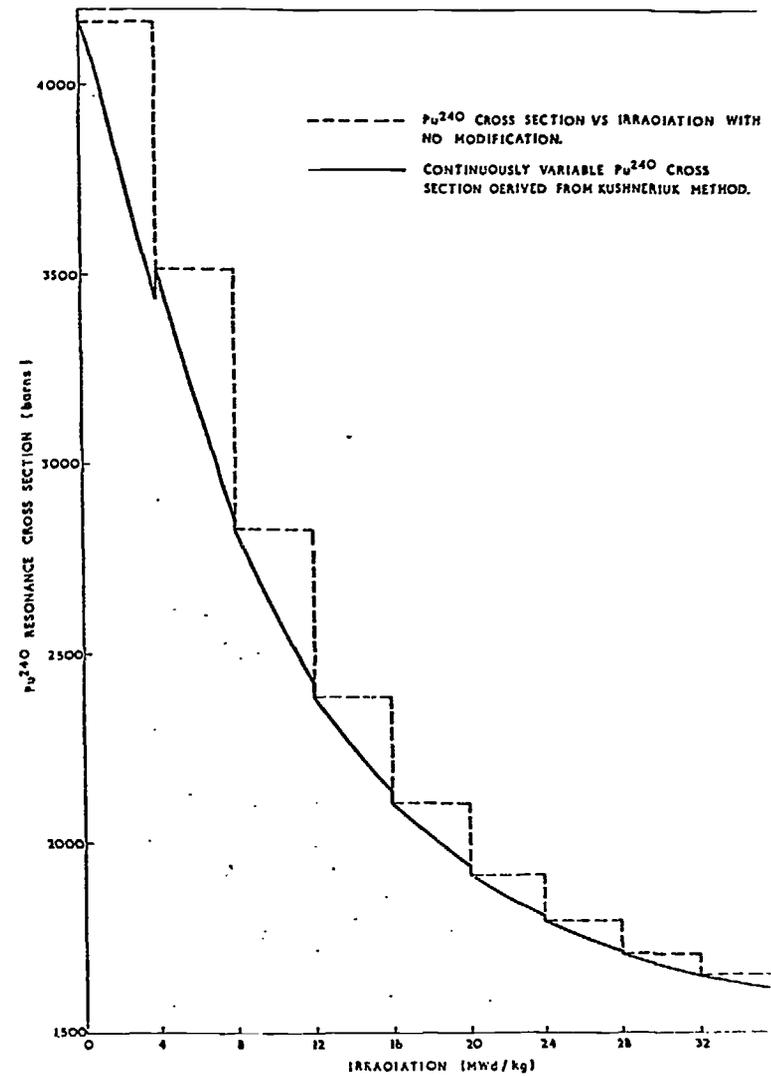
FIG. 27  $Pu^{240}$  RESONANCE CROSS SECTION VS IRRADIATION
