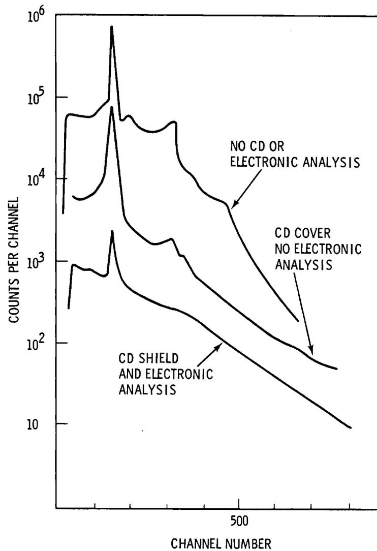
FIGURE 6.7. Effect of Cadmium Covering and Electronic Pulse Pile-Up Rejection Circuitry in Reducing the Amount of Pulse Pile-Up in High Dose Rate Neutron Fields
