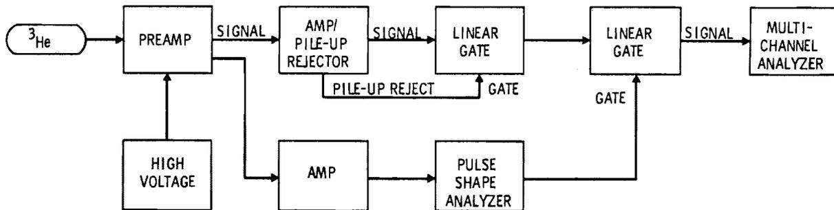
FIGURE 6.6. Block Diagram of the Electronic Equipment Used to Construct the  $^3\text{He}$  Neutron Spectrometer
