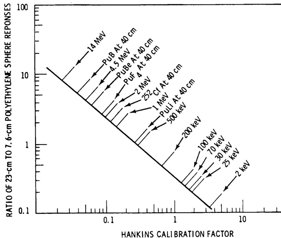
FIGURE 6.10. Effective Neutron Energy as a Function of the Ratio of 23-cm to 6.76-cm Polyethylene Sphere Responses (Griffith et al. 1979)
