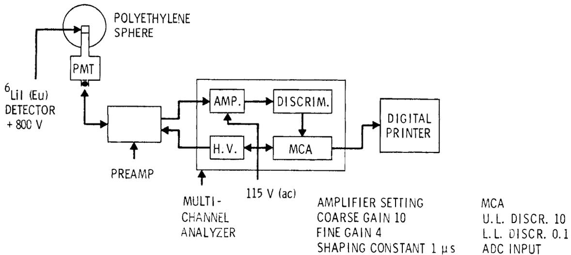
FIGURE 6.1. Block Diagram of the Multisphere System
