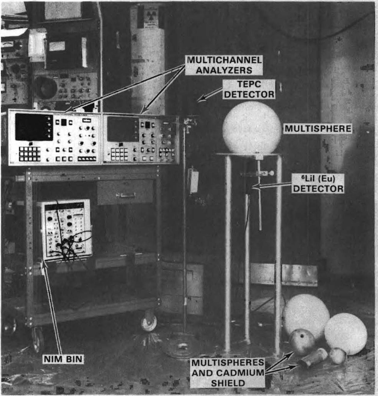
FIGURE 6.2. Multisphere Spectrometer and TEPC Systems
