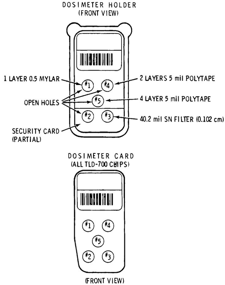
FIGURE 6.13. Modified Hanford Dosimeter for Beta Measurements
