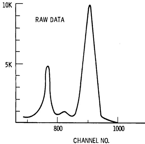
FIGURE 6.8. Results Obtained by Exposing the  $^3\text{He}$  neutron Spectrometer to 144 keV Monoenergetic Neutrons at the Filtered Neutron Beam Facility at the U.S. National Bureau of Standards
