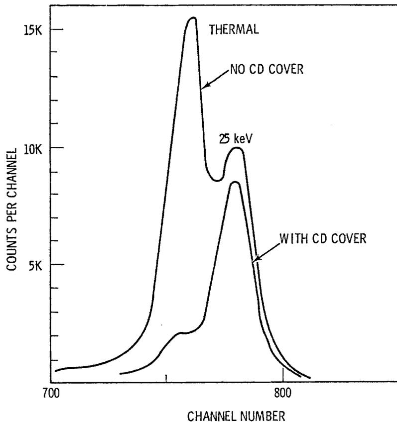
FIGURE 6.9. Results Obtained by Exposing the  $^3\text{He}$  neutron Spectrometer to 25 keV Monoenergetic Neutrons at the Filtered Neutron Beam Facility at the U.S. National Bureau of Standards
