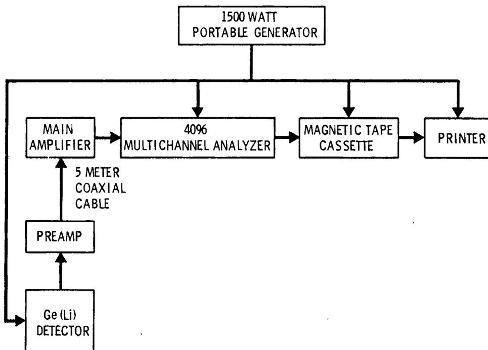
FIGURE 6.11. Simplified Layout of Equipment Used for Taking Gamma Spectrum Measurements
