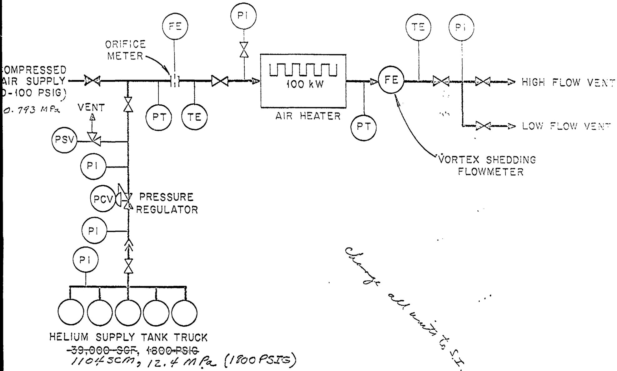
Figure 2. Test Loop Used For Remoted Sensor Signal Measurements
