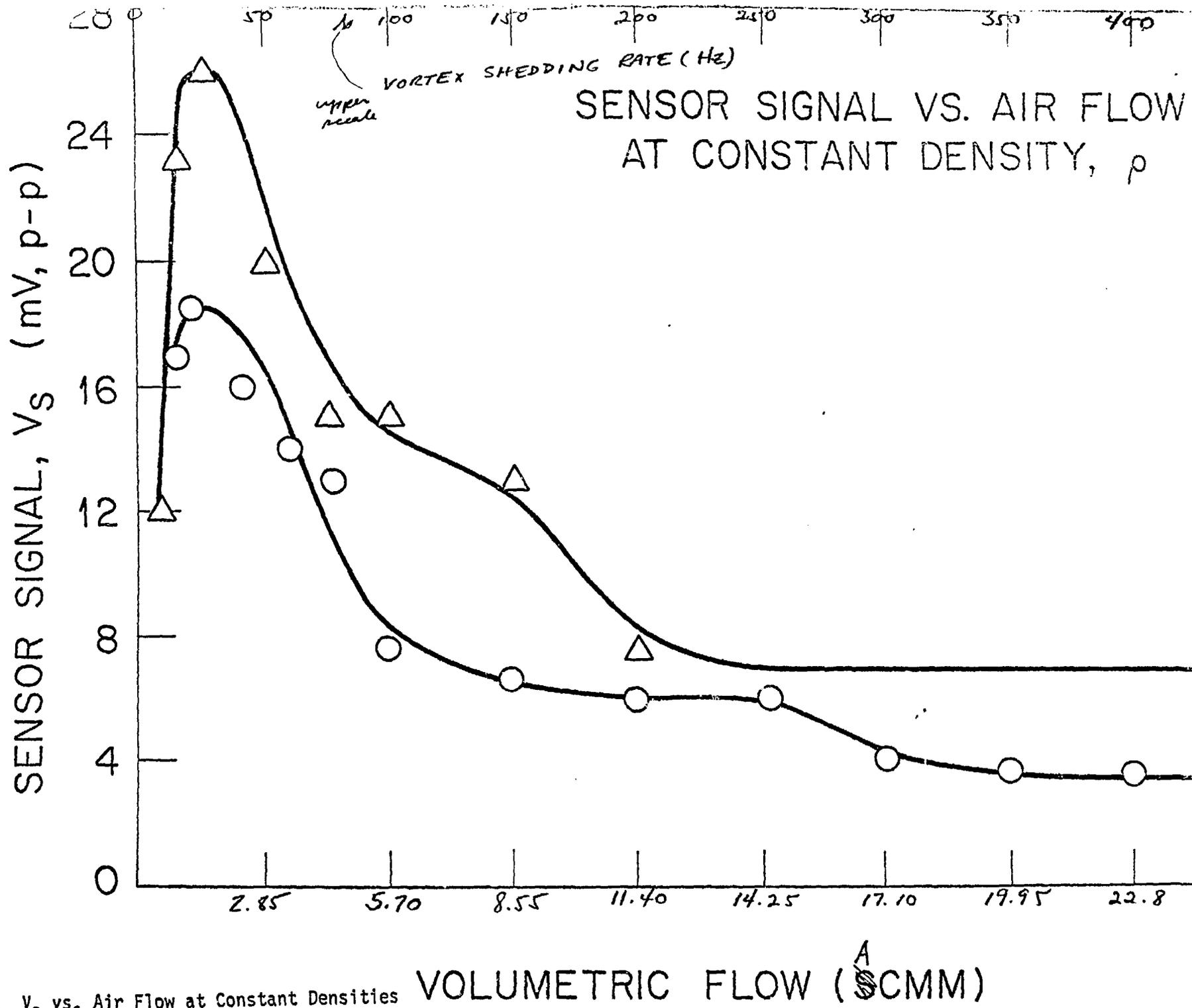
Figure 9.  $V_s$  vs. Air Flow at Constant Densities
