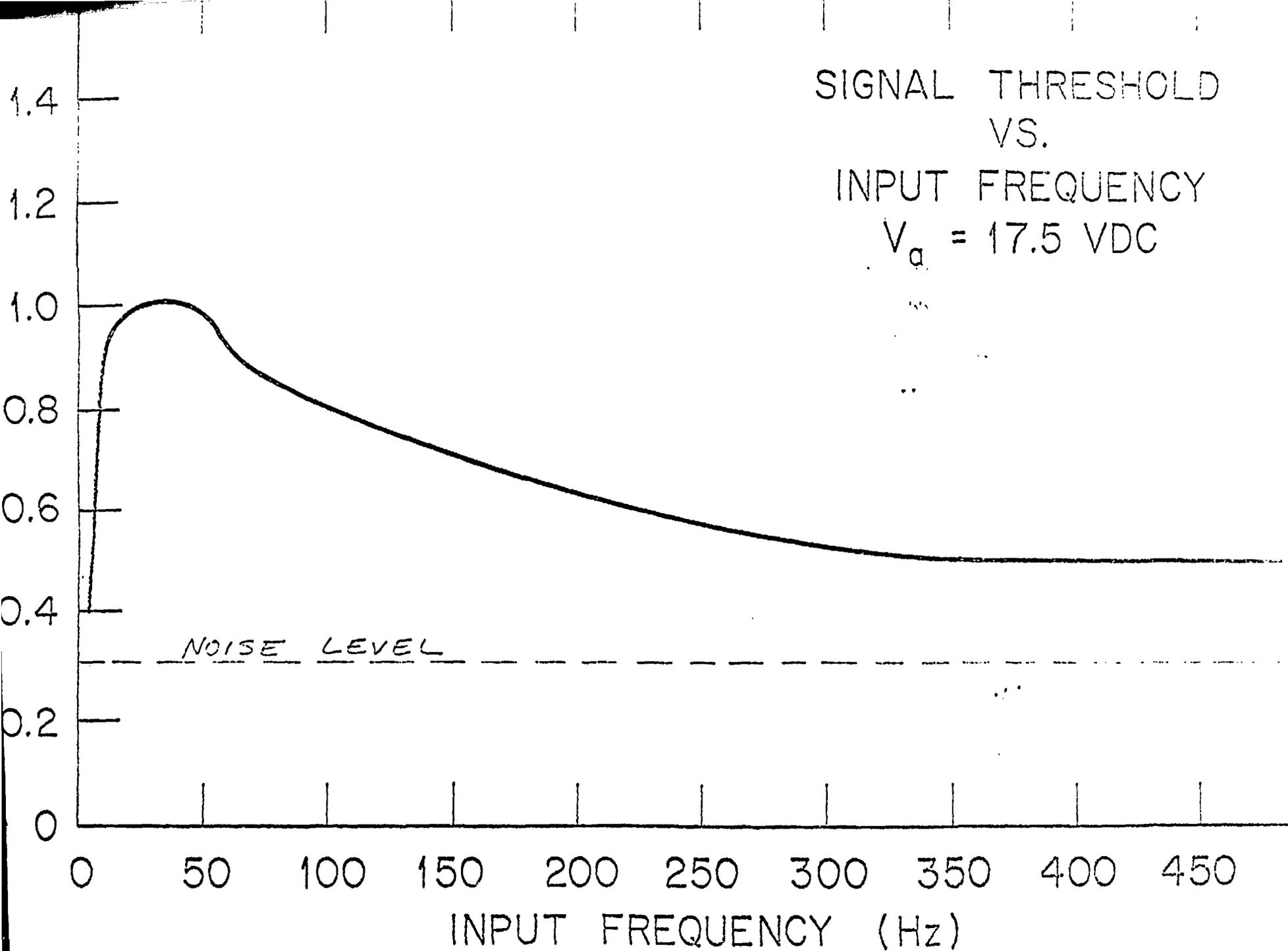
Figure 4. Signal Conditioning Electronics Threshold Response
