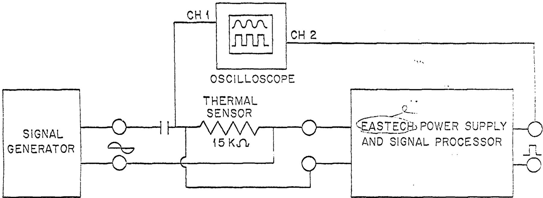
Figure 3. Block Diagram of System for Measurement of Signal Conditioning Electronics Threshold Response
