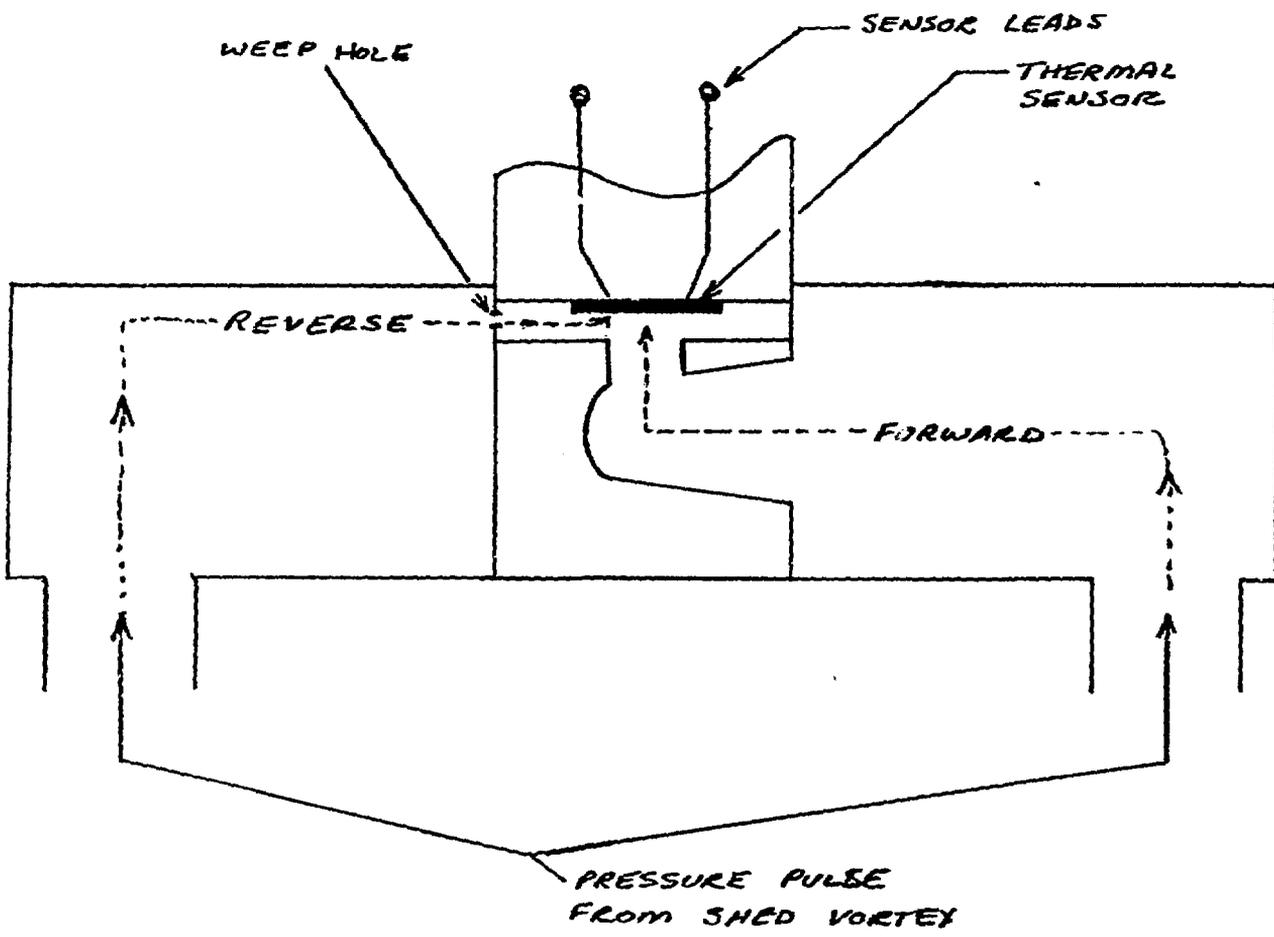
Figure 13. Schematic Diagram of Single-ported Sensor
