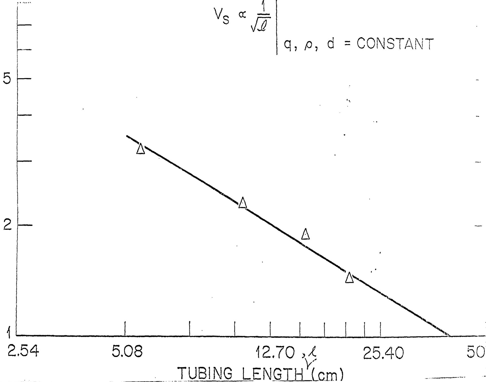
Figure 7. Relationship of  $V_S$  with Remoting Tubing Length
