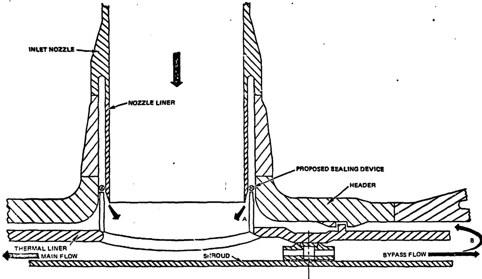
FIGURE 10. REVISED CONFIGURATION OF INLET NOZZLE REGION
