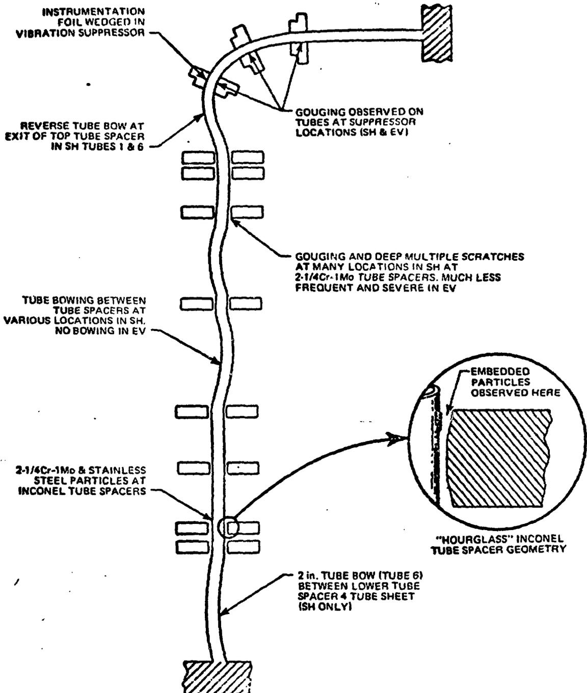
Figure 4 EVAPORATOR AND SUPERHEATER FTTM POST-TEST EXAMINATION RESULTS
