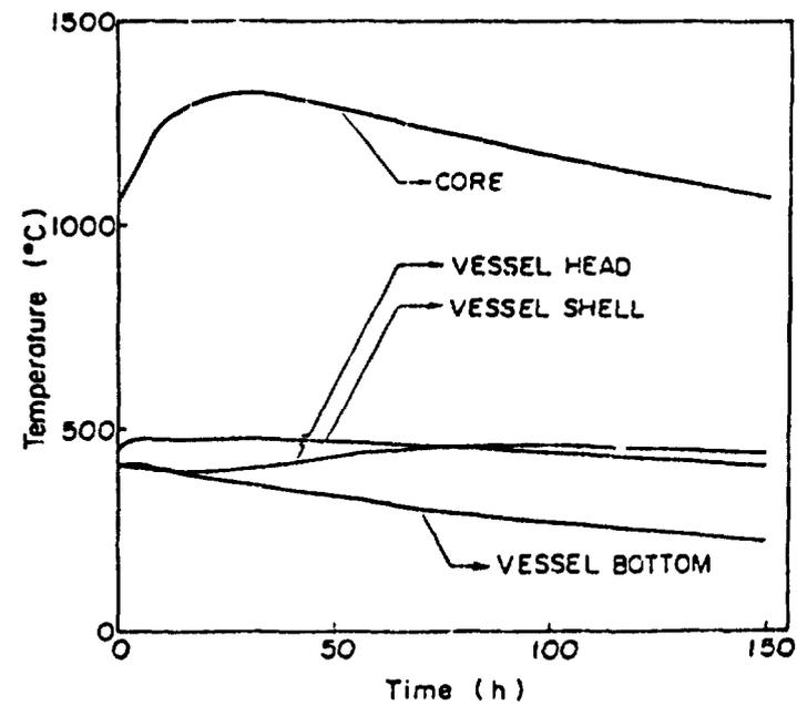
FIG. 7 TRANSIENTS OF MAXIMUM TEMPERATURE IN THE REACTOR FOLLOWING THE FAILURE OF PRIMARY COOLANT BOUNDARY
