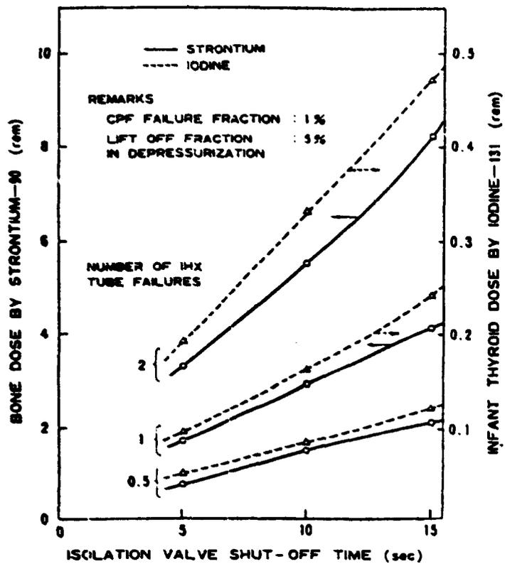
FIG. 4 DOSE AT THE SITE BOUNDARY FOLLOWING SECONDARY PIPE RUPTURE
