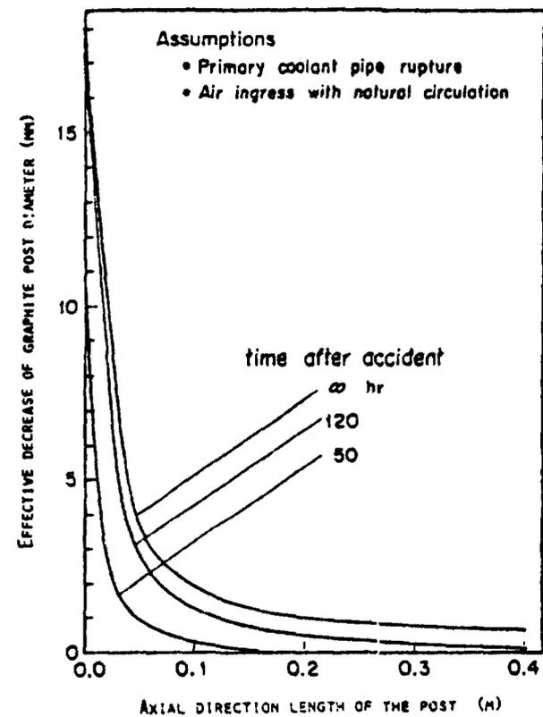
FIG. 9 AIR OXIDATION OF THE CORE SUPPORT POST GRAPHITE FOLLOWING A PRIMARY COOLANT PIPE RUPTURE
