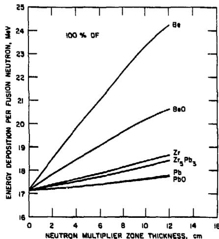
Fig. 4. Nuclear energy deposition per fusion neutron from the separate zones blanket option for the different neutron multipliers (externally cooled) with LiAlO<sub>2</sub> (90% <sup>6</sup>Li) breeder, H<sub>2</sub>O coolant, and PCA structure.
