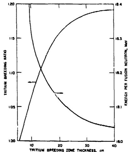
Fig. 13. Tritium breeding ratio and energy deposition per fusion neutron as a function of the breeding zone thickness with  $Zr_5Pb_3$  neutron multiplier,  $LiAlO_2$  (60%  $^6Li$ ), PCA structure, and  $H_2O$  coolant.
