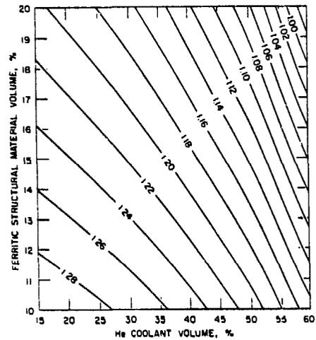
Fig. 8. Tritium breeding ratio contours for  $\text{Li}_2\text{O}$  breeder, He coolant, ferritic steel structure and  $\text{D}_2\text{O}$  first wall coolant.
