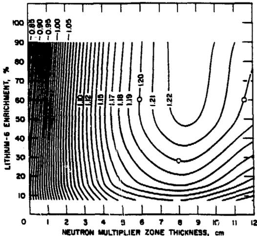
Fig. 5. Tritium breeding ratio contours for the separate zones blanket option with  $\text{LiAlO}_2$  breeder,  $\text{Zr}_5\text{Pb}_3$  neutron multiplier,  $\text{H}_2\text{O}$  coolant, and PCA structure.
