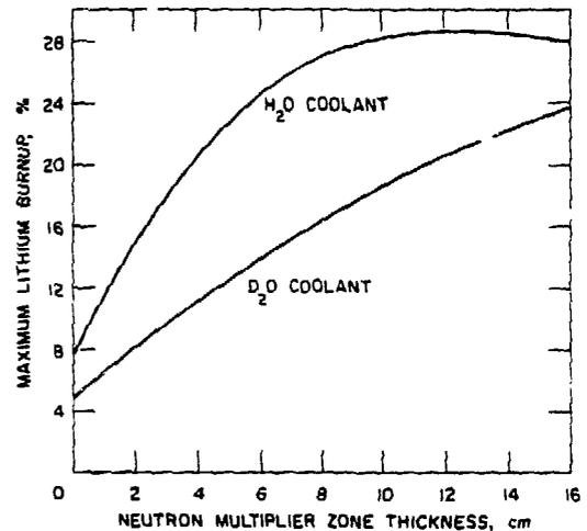
Fig. 12. Maximum lithium burnup at  $16.2 MW\text{-yr}/m^2$  as a function of the neutron multiplier zone thickness for separate zones blanket option with  $D_2O$  and  $H_2O$  coolant, lead neutron multiplier,  $Li_2SiO_3$  (90%  $^6Li$ ) breeder, and ferritic steel structure.
