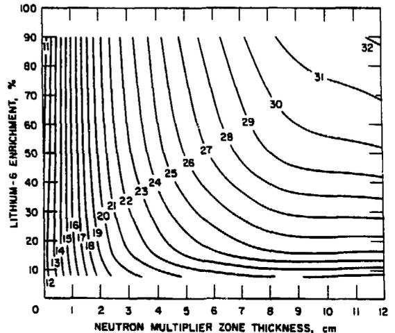
Fig. 7. Maximum lithium burnup (%) contours after six years of operation ( $16.2 \text{ MW}\cdot\text{yr}/\text{m}^2$ ) for the separate zones blanket option with  $\text{LiAlO}_2$  breeder,  $\text{Zr}_5\text{Pb}_3$  neutron multiplier,  $\text{H}_2\text{O}$  coolant, and PCA structure.
