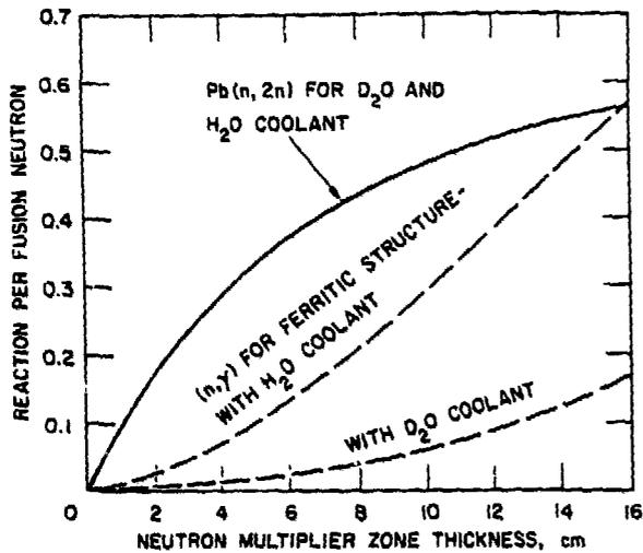
Fig. 10.  $Pb(n,2n)$  neutron interaction and  $(n,\gamma)$  capture in the ferritic structure for  $D_2O$  and  $H_2O$ -cooled blanket with  $Li_2SiO_3$  (90%  $^6Li$ ) breeder.
