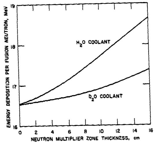
Fig. 11. Nuclear energy deposition per fusion neutron from separate zones blanket option with  $D_2O$  and  $H_2O$  coolant, lead neutron multiplier,  $Li_2SiO_3$  (90%  $^6Li$ ) breeding and ferritic steel structure.
