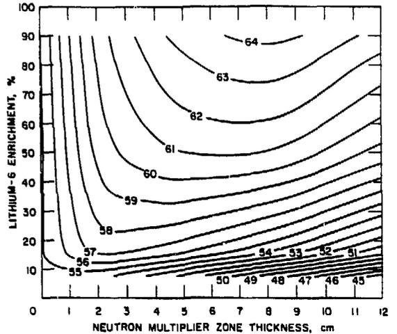
Fig. 6. Maximum heating rate ( $\text{W}/\text{cm}^3$ ) contours for the separate zones blanket option with  $\text{LiAlO}_2$  breeder,  $\text{Zr}_5\text{Pb}_3$  neutron multiplier,  $\text{H}_2\text{O}$  coolant, and PCA structure.
