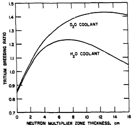
Fig. 9. Tritium breeding ratio from separate zones blanket option with D<sub>2</sub>O and H<sub>2</sub>O coolant, lead neutron multiplier, Li<sub>2</sub>SiO<sub>3</sub> (90% <sup>6</sup>Li) breeder, and ferritic steel structure.
