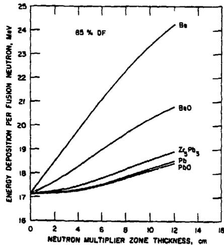
Fig. 2. Nuclear energy deposition per fusion neutron from the separate zones blanket option for the different neutron multipliers (internally cooled) for LiAlO<sub>2</sub> (90% <sup>6</sup>Li) breeder, H<sub>2</sub>O coolant, and PCA structure.
