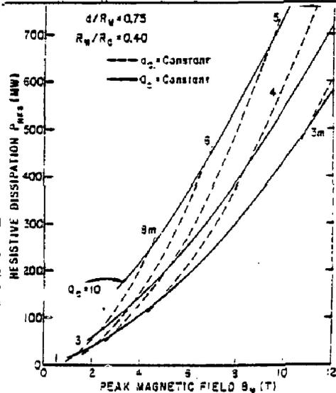
Fig. 3. Variation of  $P_{res}$  with field at conductor  $B_M$  and fusion electrical power gain  $Q_c$ .
