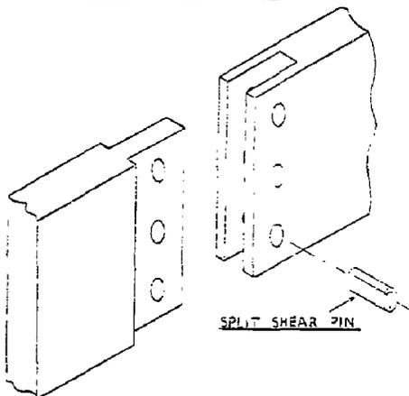
Fig. 8. Details of the lap joint for the configuration of Fig. 6.
