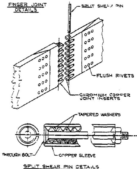
Fig. 7. Details of the finger joint for the configuration of Fig. 6.
