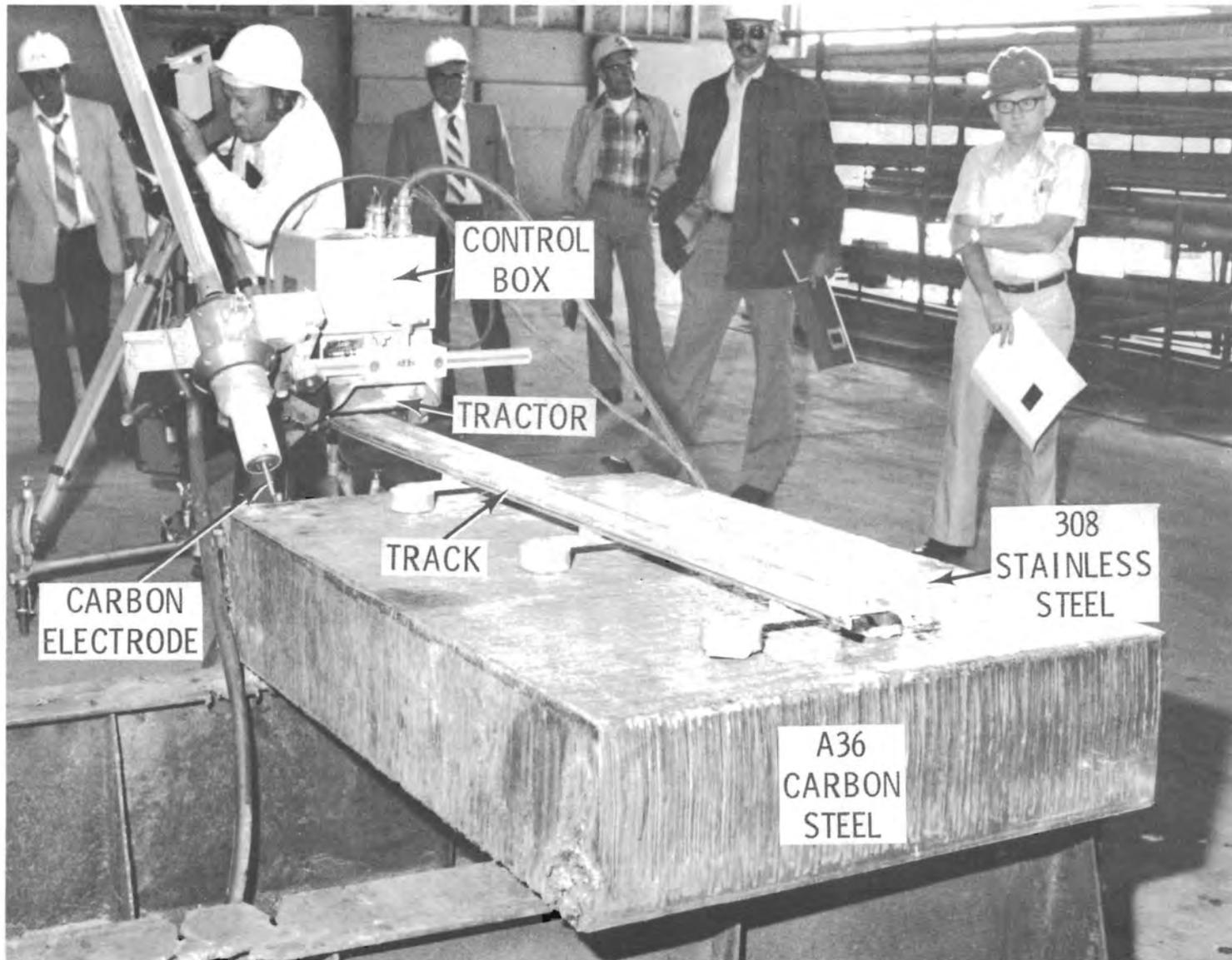
FIGURE 5. Test Arrangement With Arc Gouger in Place
