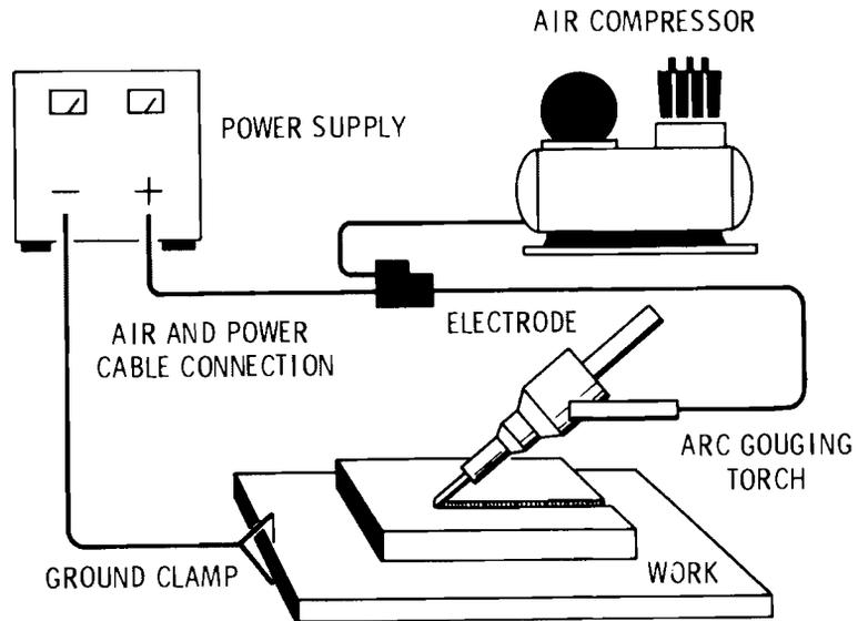
**FIGURE 3.** Schematic of Air Arc Gouging Technique
