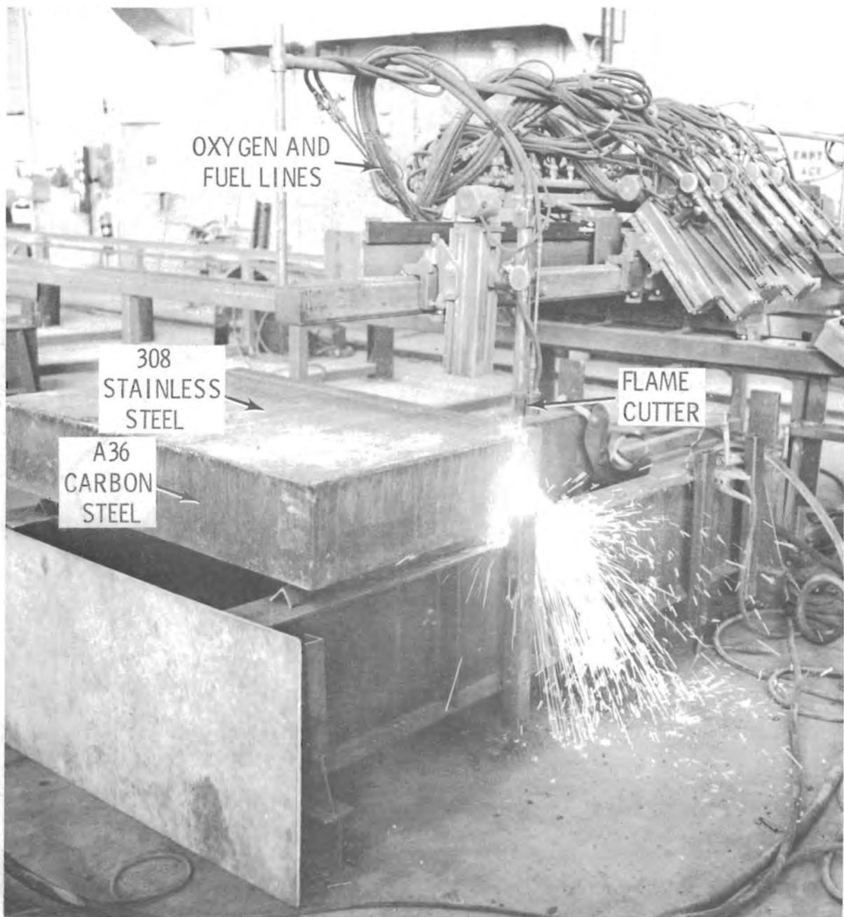
FIGURE 9. Initiation of the Flame Cutting Procedure
