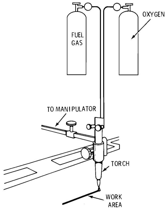
FIGURE 4. Schematic of Flame Cutting Equipment
