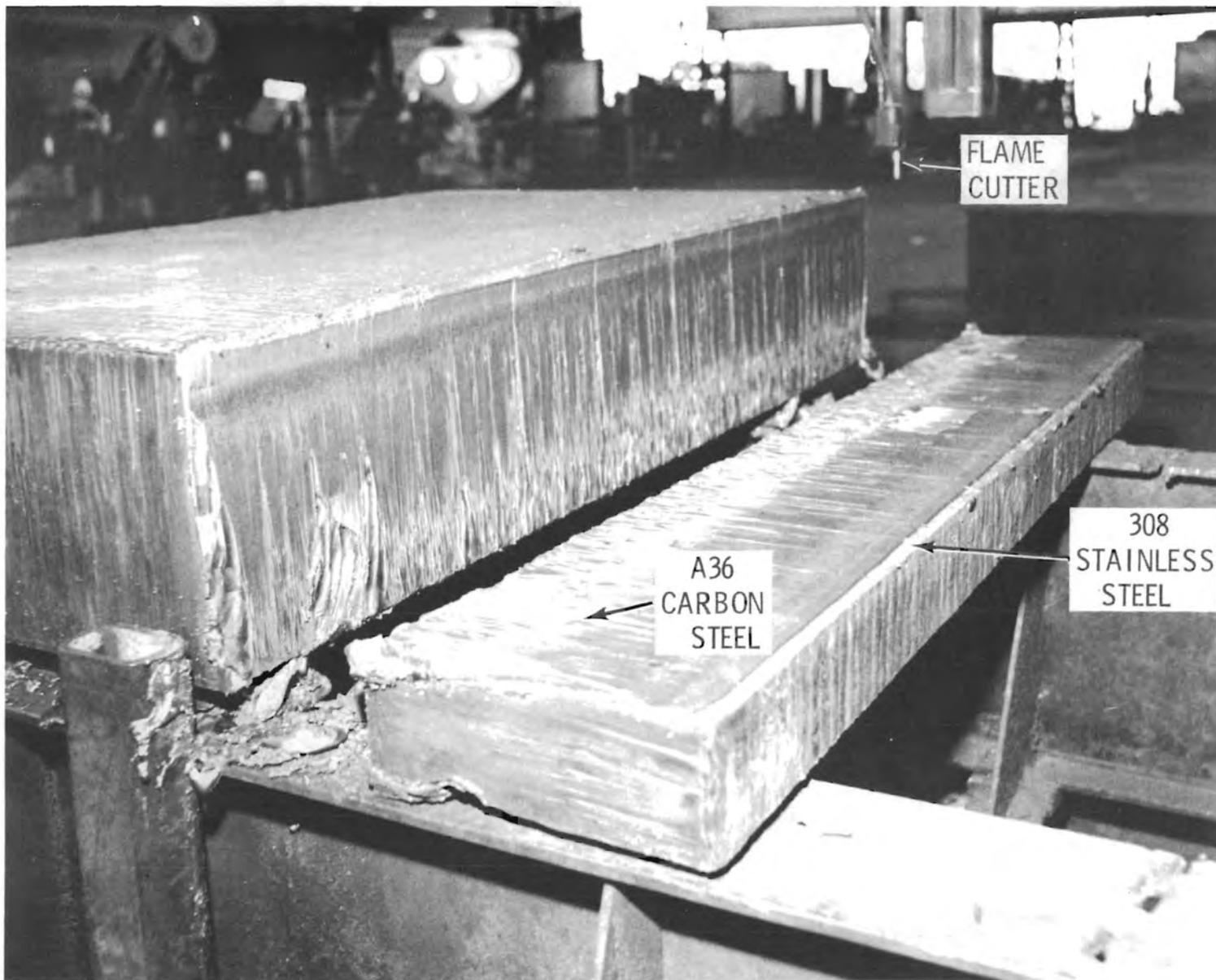
FIGURE 10. View of Completely Severed Sample
