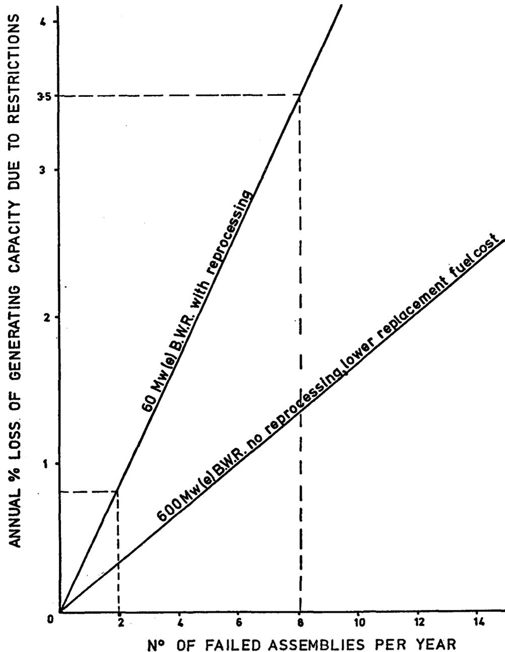
**FIG. 5. BREAK-EVEN RELATIONSHIP BETWEEN COST OF FAILURES AND COST OF RESTRICTIONS**
