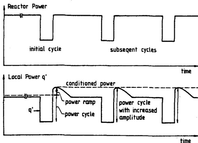
Fig. 3 The Effect of Load Follow Operation on Fuel Duty (daily or weekly cycles)
