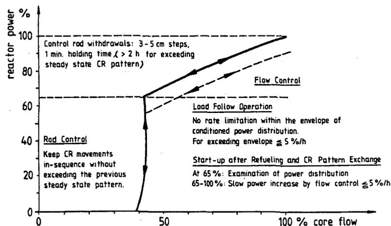
Fig. 2 KWU-BWR Operating Recommendations (prepressurized 8x8 fuel)
