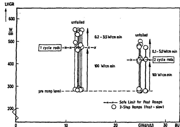
Fig. 1 Ramp Tests in HFR Petten. Ramp Power vs. Burnup (Ref. /2/). (PWR-Rods, prepressurized; Status Jan. 1979)
