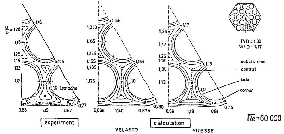
Fig. 14: Fully developed velocity distribution in 19 rod bundle (Re = 60 000; P/D = 1.30; W/D = 1.17)
