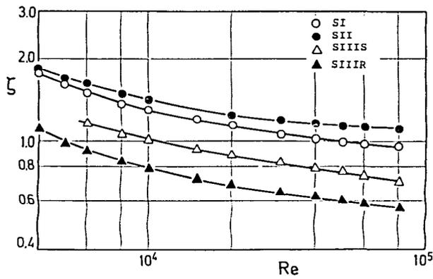
Fig. 7: Drag coefficients of various grid type spacers
