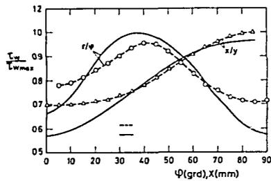
Fig. 13: Comparison of the measured wall shear stress distributions in the wall channel (P/D = 1.07) with VELASCO-results
