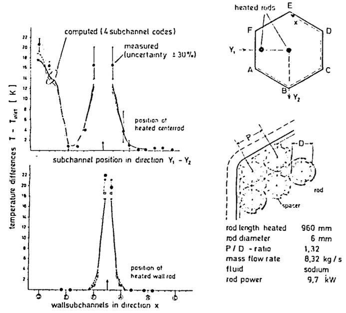
Fig. 5: Mean subchannel temperatures: Comparison between computed and experimental results /14/
