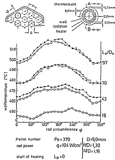
Fig. 18: Temperature distribution in 19-rod bundle at the circumference of the side rod ( $Pe = 170$ ;  $P/D = 1.3$ ;  $W/D = 1.19$ ;  $q = 104\text{ W/cm}^2$ )
