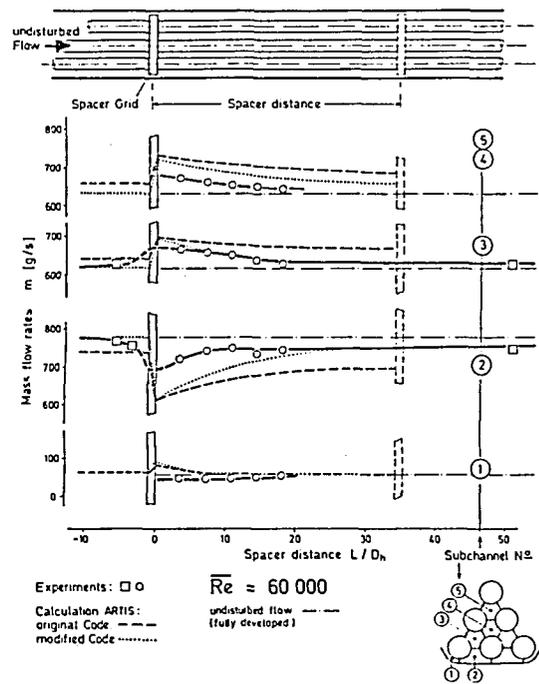
Fig. 16: Mass flow distribution in 19 rod-bundle with grid spacer ( $Re = 60\,000$ ;  $P/D = 1.30$ ;  $W/D = 1.17$ )
