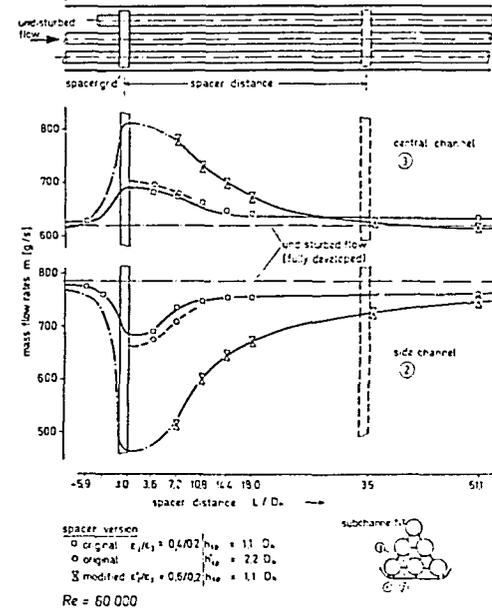
Fig. 17: Mass flow distribution in 19-rod bundle with varying grid spacer blockages and grid heights ( $Re = 60\,000$ ;  $P/D = 1.3$ ;  $W/D = 1.17$ )
