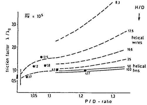
Fig. 8: Friction factors as function of P/D and H/D-ratio for 61 rod bundles wire helical spacer types (37/61-rod bundles)
