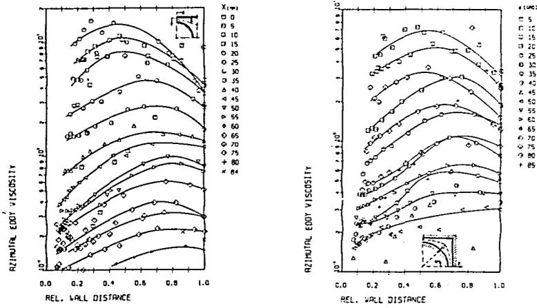
Fig. 12: Dimensionless eddy viscosity parallel to the channel wall in the wall channel (P/D = 1.07) and corner channel (W/D = 1.07) as a function of the dimensionless distance from the wall
