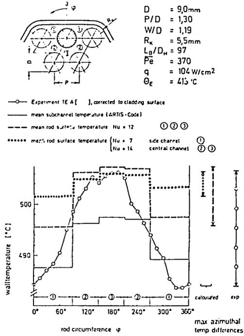
Fig. 21: Azimuthal temperature variation of the side rod cladding: Comparison between local measurements - global calculations
