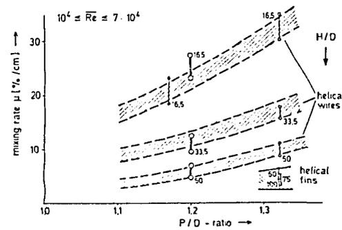
Fig. 9: Mixing coefficients as function of P/D and H/D-ratio for 61-rod bundles with helical spacer types
