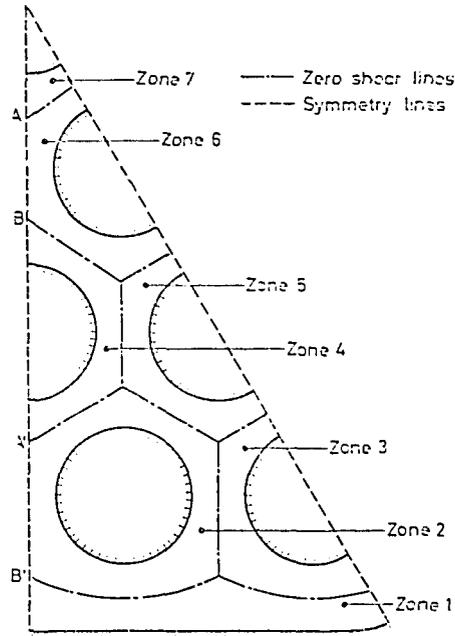
Fig. 3: Qualitative picture of the zero shear lines in a subarray representative for a thirty-seven rod array
