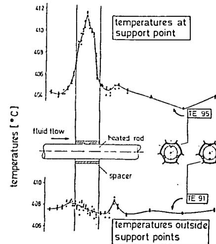
Fig. 19: Axial temperature distribution of a rod in the spacer region ( $Pe = 346$ ;  $P/D = 1.3$ ;  $W/D = 1.19$ ;  $q = 73\text{ W/cm}^2$ ;  $L_B/D_H = 97$ )
