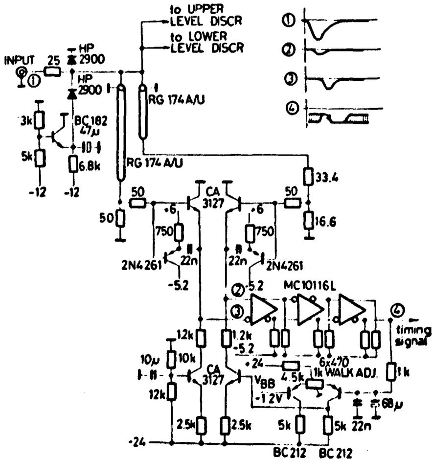
Fig. 11 Circuit diagram of the constant-fraction block
