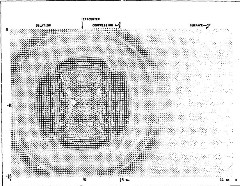
FIGURE 4: SEISMIC WAVES RADIATING OUTWARD DUE TO VERTICAL "RUPTURE" AT HYPOCENTRE (Time =  $T_1 + 2\frac{1}{2}$  Sec.)
