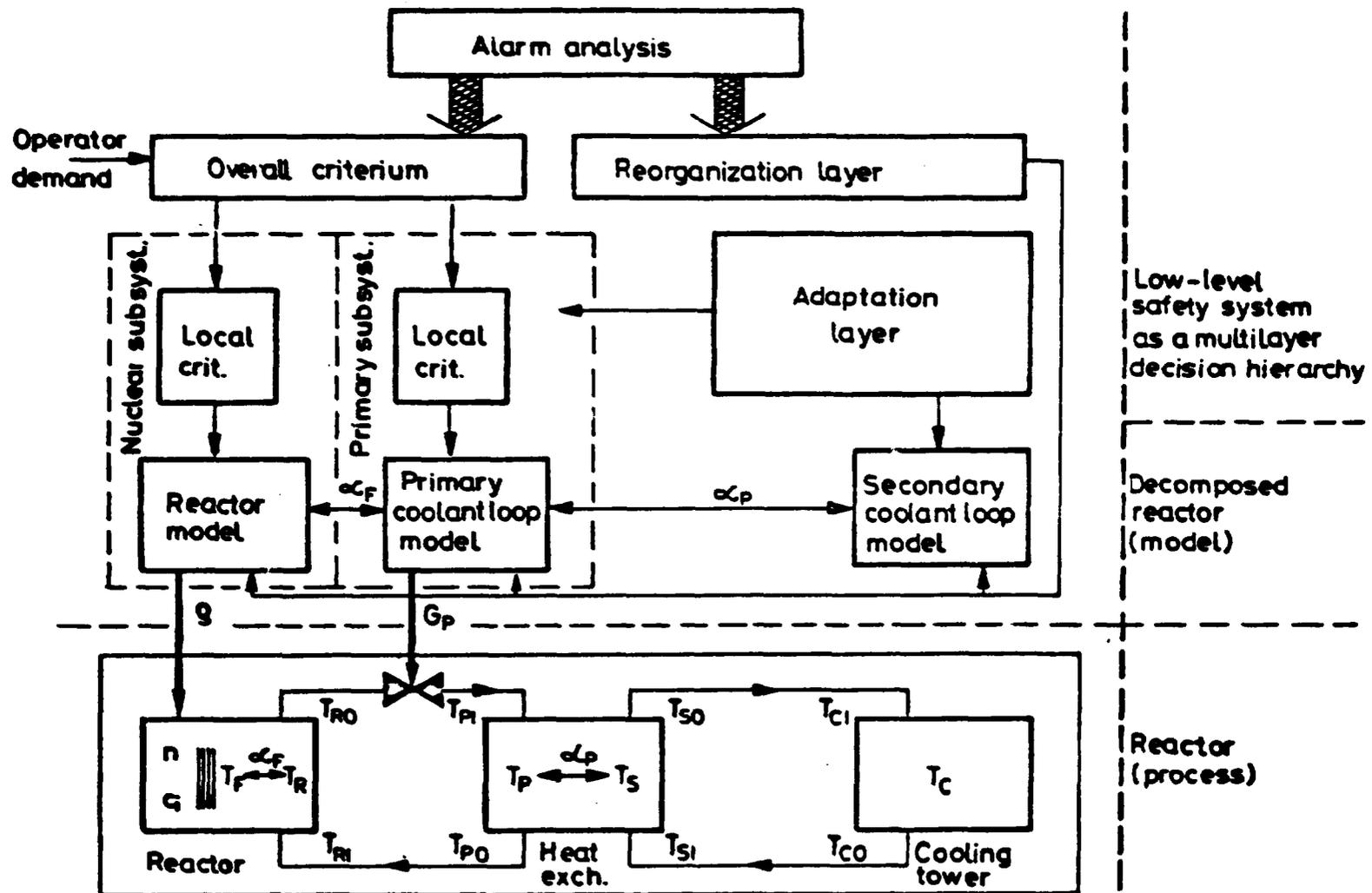
upper level of the hierarchy, takes into account the signals of the alarm analysis and determines the operational status of the process /i.e. normal, emergency, etc./ and on the basis of the decision it selects the relevant model and control algorithm.
