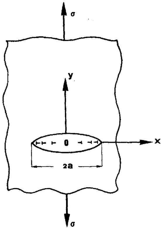
Fig.1 The crack dislocation model.
