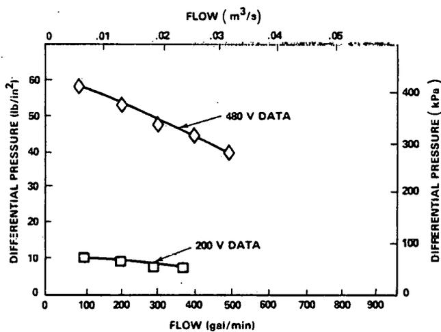
FIGURE 4. ALIP 600-30 Performance at  $2.7 \times 10^{-1}$  Pa in Surge Tank and Solid-State Controls. Neg 8108183-1
