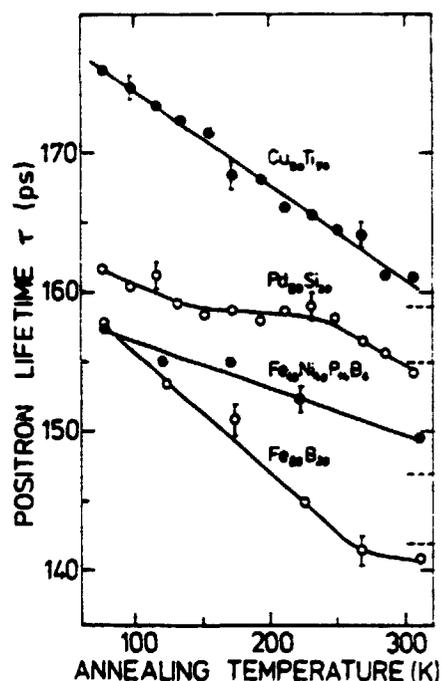
Fig. 1. Positron lifetime as a function of isochronal annealing temperature in various amorphous alloys electron irradiated at 20 K. Dotted lines in the right margin of the figure represent positron lifetime values in the as-received state of the corresponding alloys.
