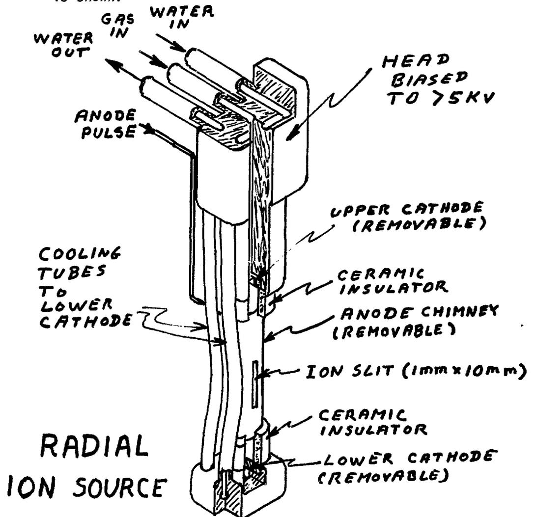
After about 4 months of operating experience with this prototype, a new ion source was constructed. The new design simplifies the regular servicing procedures and also provides better protection against electrical discharges of the source to ground due to the d.c. bias. This new ion source is now the regular source for alpha particle beam operation.
