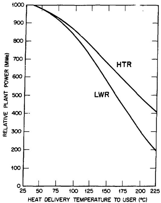
**Fig. 2. Approximate Variation of Plant Output with Temperature of Delivered Bottom Energy. (Based on Information from J. M. Neill, Advanced Energy Concepts, Feb. 1981)**
