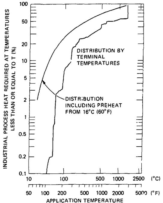
Fig. 1. Cumulative Distribution of Process Heat Requirements (6) (1976 estimate)
