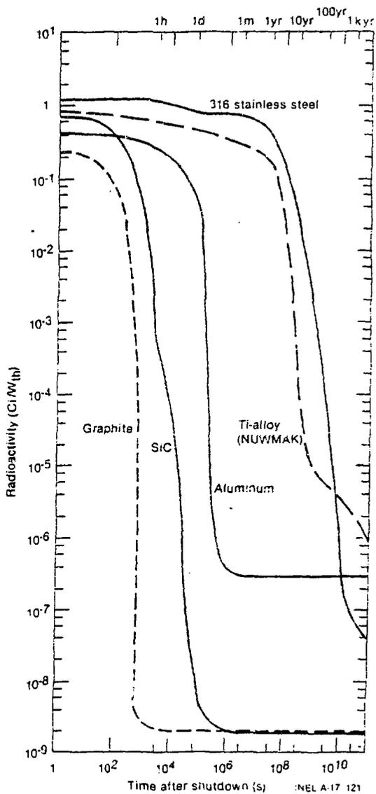
Figure 2. Postshutdown radioactivities for several fusion reactor first wall-blanket structures after two years of operation at  $1.5 \text{ MW/m}^2$  neutron wall loading.
