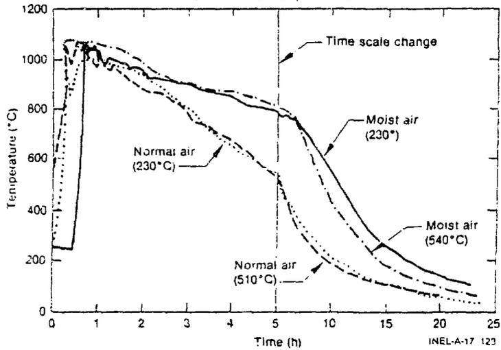
Figure 3. Lithium pool reaction in air. (Conditions: 10 kg lithium at 230, 510, and 540°C; 0.2-m<sup>2</sup> pool in 14-m<sup>3</sup> vessel.)
