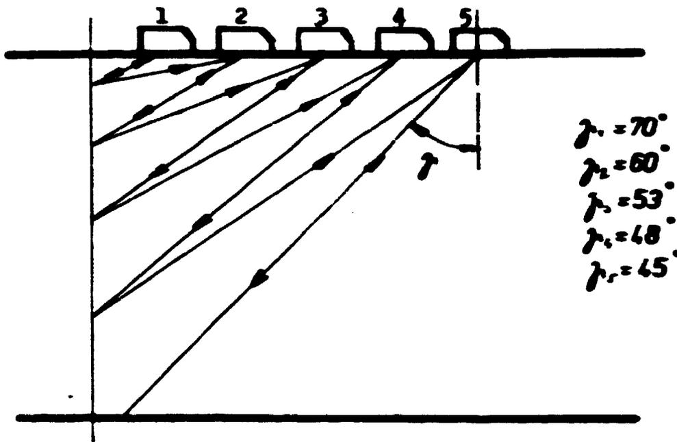
**Fig. 5. Tandem for direct reflection**
