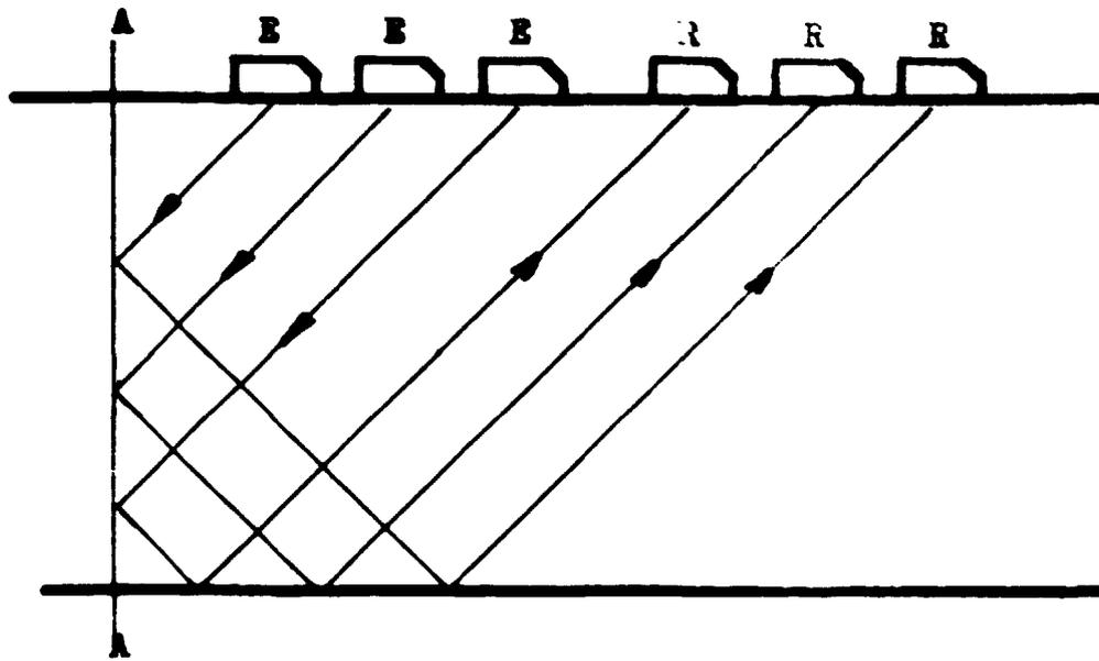
Fig. 3. Tandem for indirect reflection
