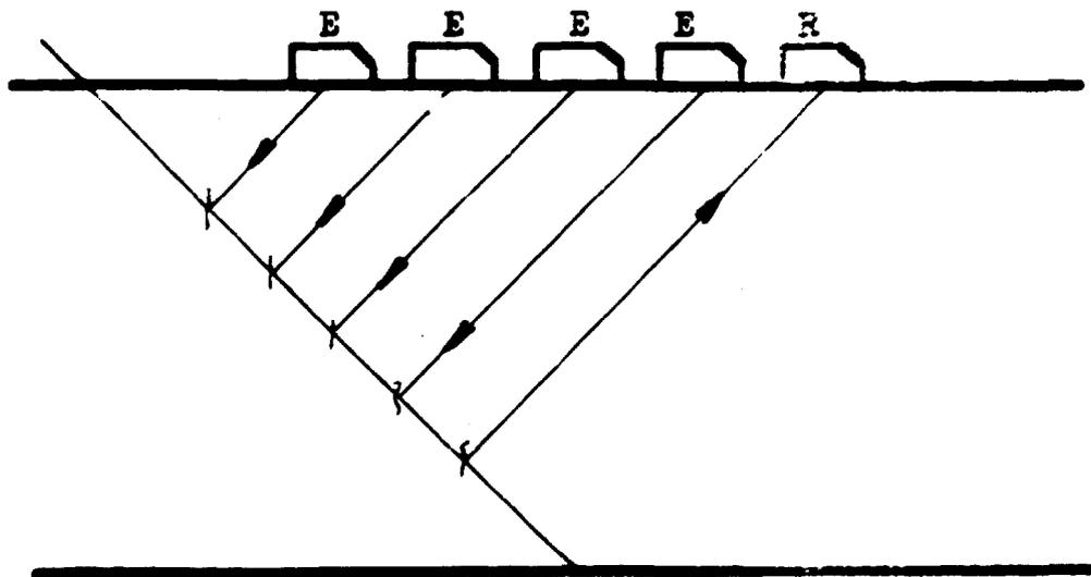
Fig. 4. Tandem for indirect reflection
