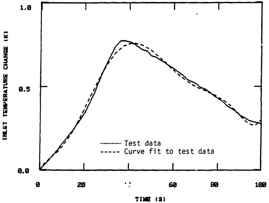
Figure 5. Steam generator water level controller setpoint decrease; reactor inlet temperature response
