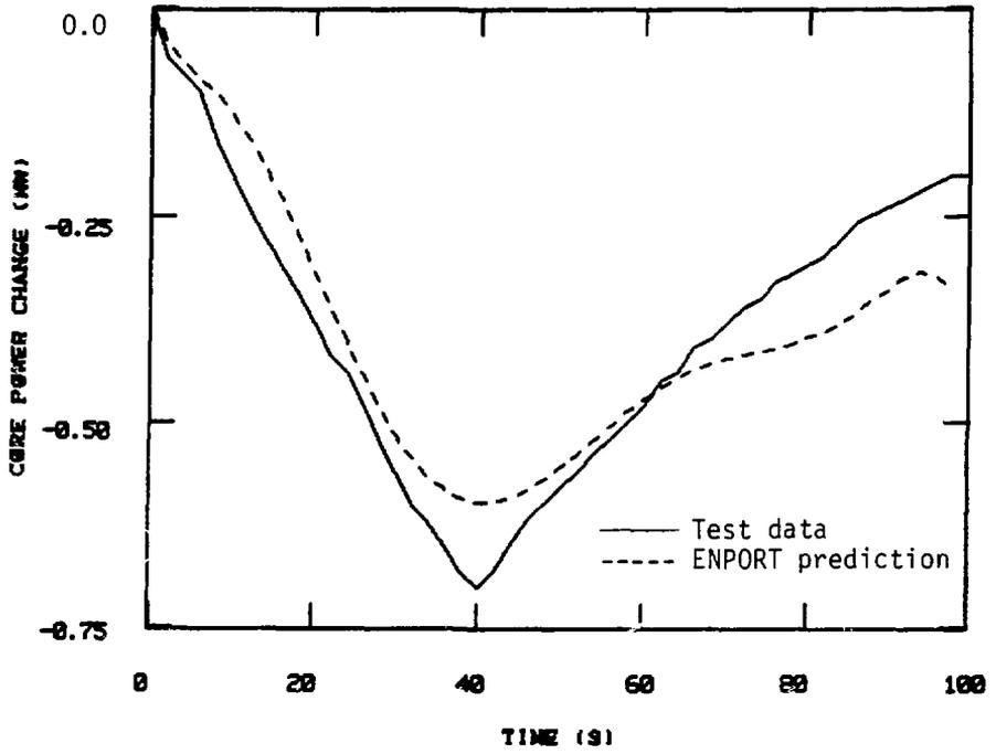
Figure 7. Steam generator water level controller setpoint decrease; core power response
