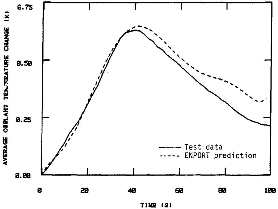
Figure 6. Steam generator water level controller setpoint decrease; core coolant average temperature response
