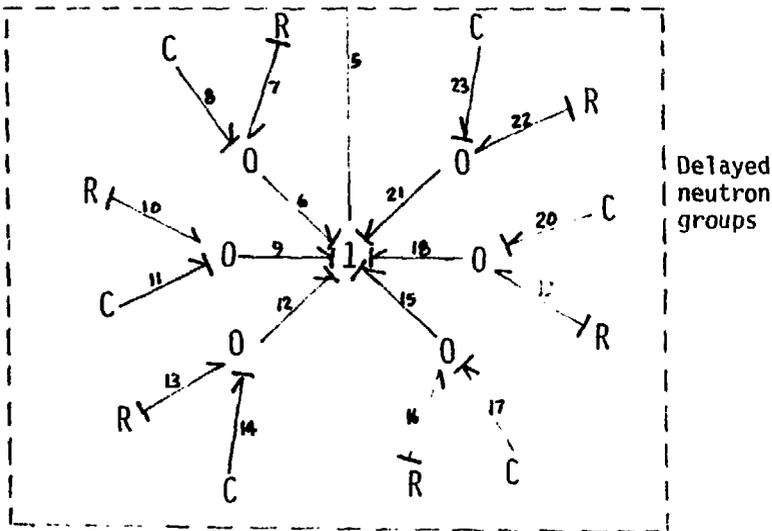
Figure 4. Bond graph representation of nuclear reactor dynamics
