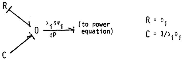
Figure 2. Pseudo-bond graph of delayed neutron group equation
