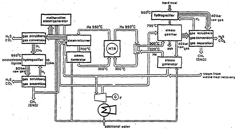
FIG. 5 FLOW SCHEME OF PNP 500 MW
