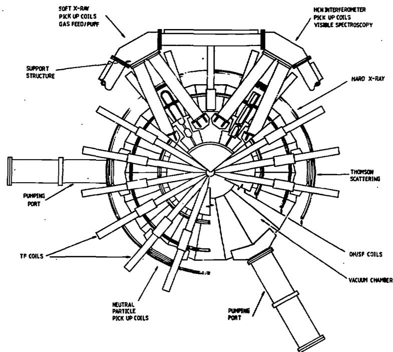
FIG. 1. Layout of machine and diagnostics
