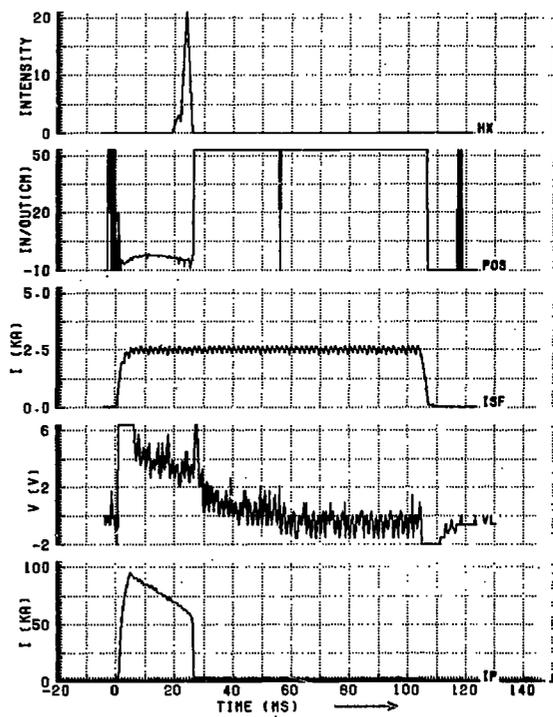
FIG. 2. Some typical data for a Tokamak discharge. The traces from top to bottom are hard X-ray flux (HX), horizontal position (POS), shaping field current (ISF), loop voltage (VL) and plasma current (IP).
