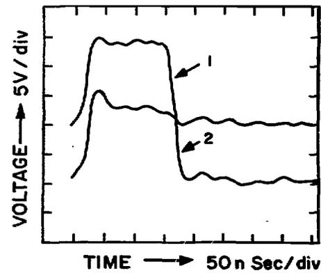
Fig. 2: Current pulse shape (1) and the shape of resulting magnetic field (2).
