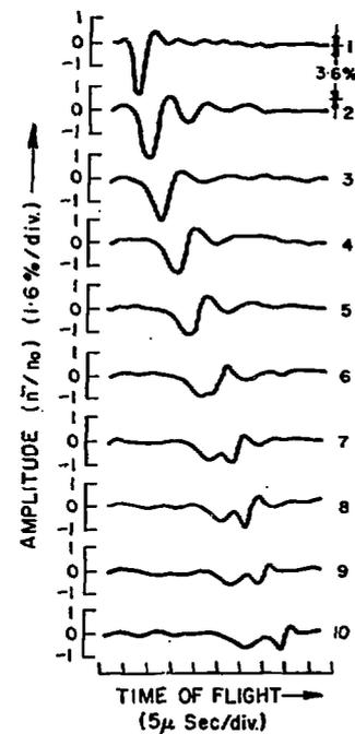
Fig. 2 Typical example of rarefaction pulse propagation in the plasma. Successive traces (1 to 10) are time records taken at axial position separated by  $12.5\lambda_D$ . Horizontal axis is time of flight in  $5\mu$  sec/div and vertical axis gives amplitude ( $\frac{\delta n}{n_0}$ ) in 1.6% per division. Amplitude of step pulse applied to grid for all the traces is 1 volt.
