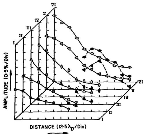
Fig. 5 Amplitude vs. axial position for rarefactive pulses of different initial amplitudes. Cases 1 to VI correspond to cases I to VI of Fig. 4 (a). Open points represent the amplitude of the original pulse and the darkened points denote the amplitude of new trough created after the fissioning.
