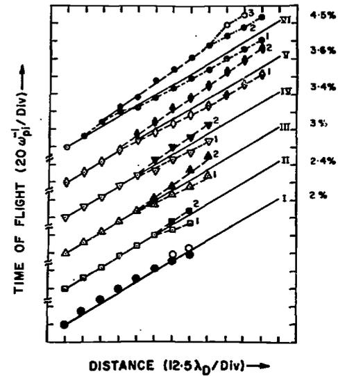
Fig. 4 Time of flight vs. Axial position for the rarefactive pulses of different initial amplitudes 2% to 4.5%. The initial amplitudes are indicated on right hand side.
