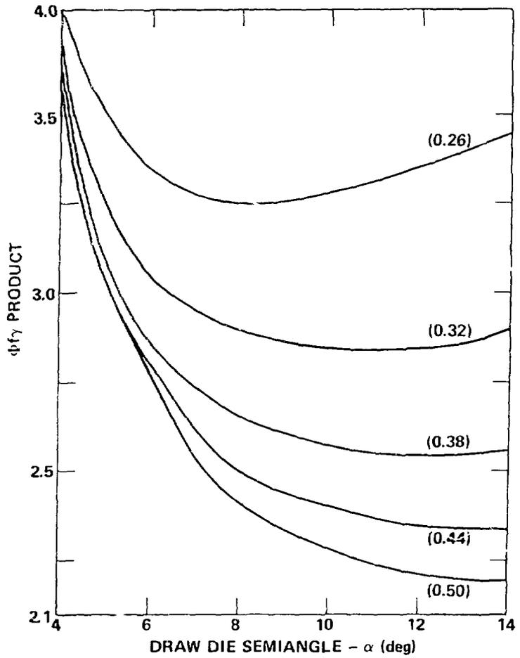
Fig. 9.  $\phi\gamma$  product vs draw-die semiangle at various amounts of cold work ( $\mu = 0.19$ ).
