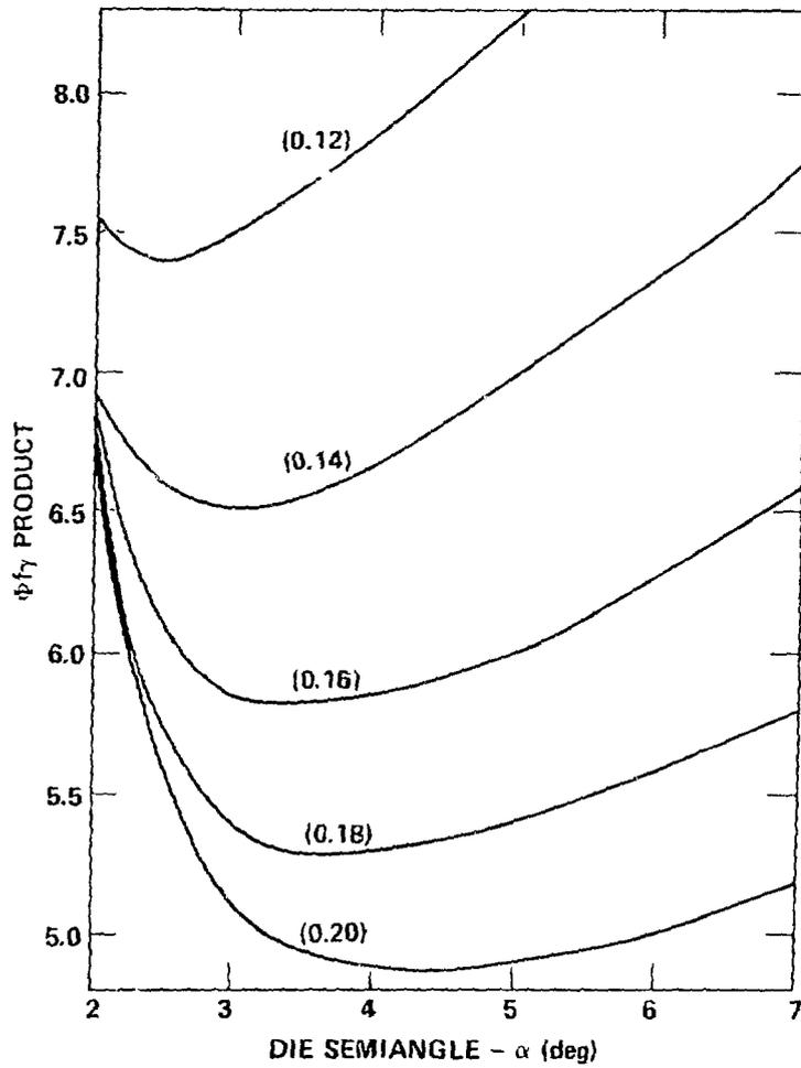
Fig. 10.  $\Phi f_y$  product vs draw-die semiangle for various amounts of second-draw cold work ( $\mu = 0.19$ ).
