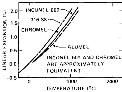
Fig. 3. Average linear thermal expansion of materials for CFTL FRS cladding and thermocouple components.
