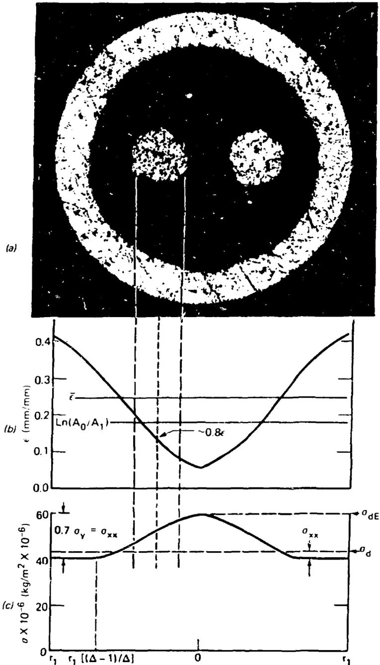
Fig. 8. A schematic representation of radial stress and strain pattern across a thermocouple drawn with  $\Delta = 3$  and  $\epsilon = 0.17$ . Average strain is increased to  $\bar{\epsilon}$  by nonuniform distribution, and strain of thermocouple is about  $0.8\epsilon$ . Internal stress is maximum in the center and depends on yield stress as well as  $\Delta$ .
