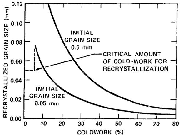
Fig. 4. Schematic curves of recrystallized grain size vs amount of cold work before recrystallization.
