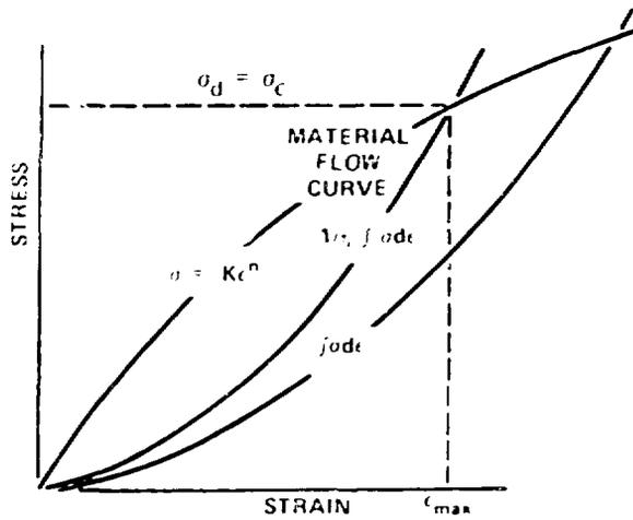
Fig. 7. Flow-curve ( $K\epsilon^n$ ) for a solid wire that exhibits strain hardening as well as work curve for ideal ( $\int \sigma d\epsilon$ ) and typical ( $1/\eta \int \sigma d\epsilon$ ) drawing process.
