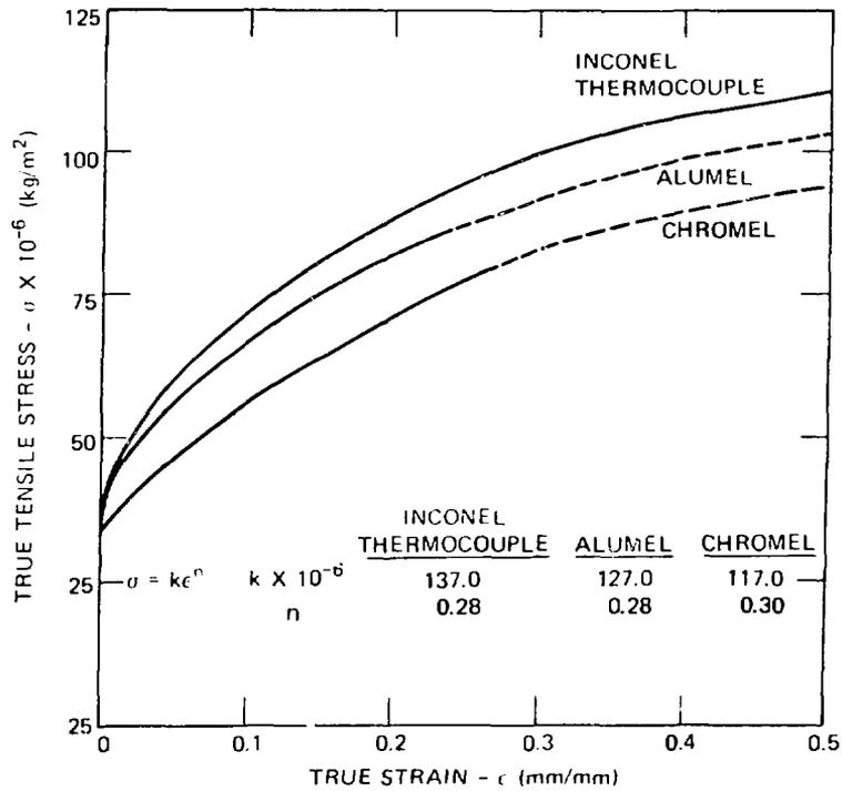
Fig. 11. True stress vs true strain for an Inconel-sheathed Type K thermocouple and for Chromel and Alumel thermoelements.
