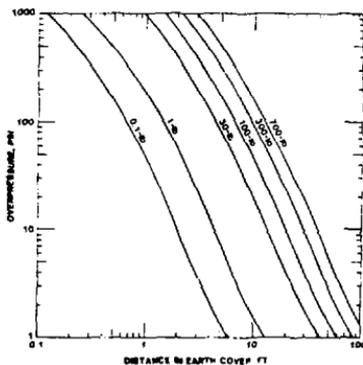
Figure 1. Overpressure in Earth Cover vs Distance from the Explosive (Ref 3)
