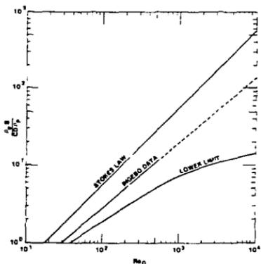
Figure 2. Particle Travel Distance vs Reynolds Number
