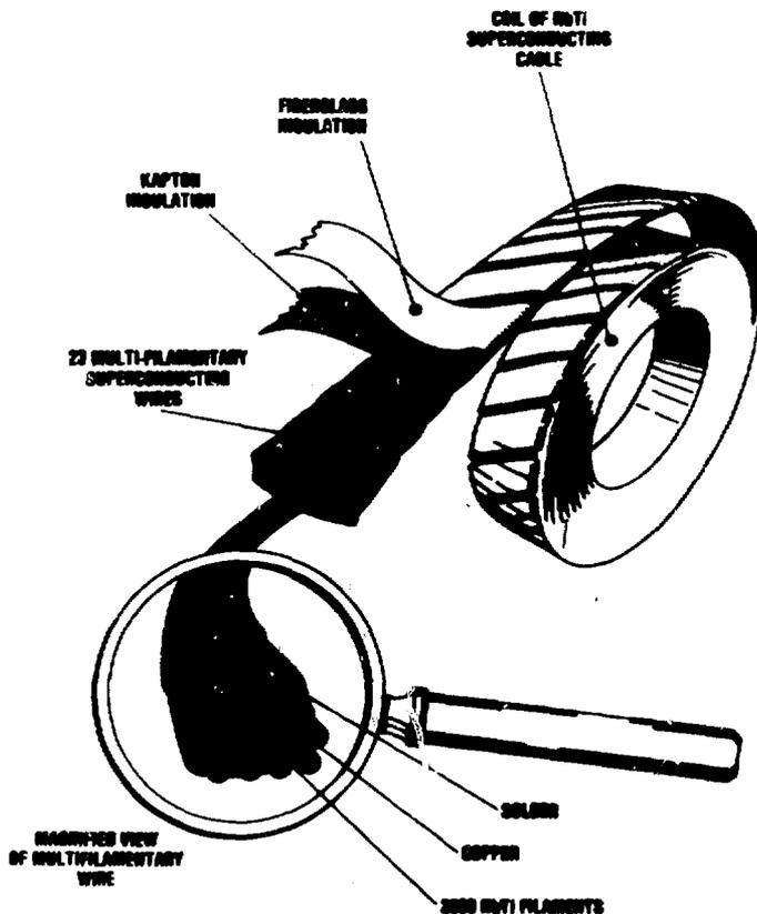
Figure 2. Schematic drawing of 23-strand superconducting cable. The cable is approximately 0.78 cm wide.
