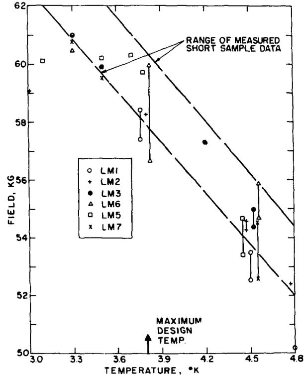
Figure (b) Quench field vs. bath temperature for dipoles LM1,2,3,5,6, and 7.
