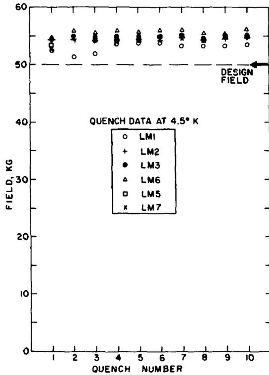
Figure (a) Training curves for dipoles, LM1,2,3,5,6, and 7, for a bath temperature of 4.5°K.
