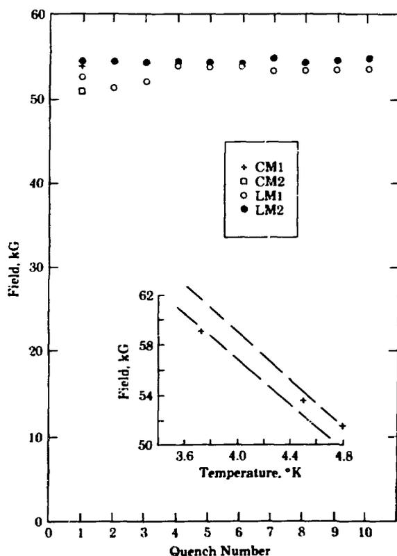
Figure 8. Training curve for four dipoles, at a bath temperature of 4.5K. The insert shows average quench field versus bath temperature for one of the magnets.
