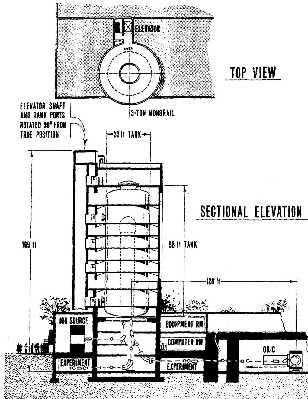
Fig. 9. Cross-sectional view of the Holifield Facility.
