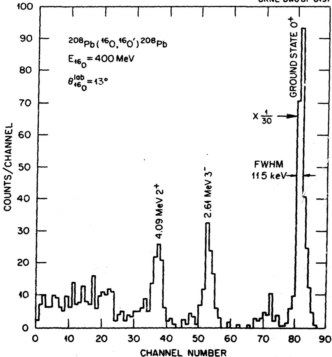
Fig. 11. A spectrum of oxygen ions scattered from a lead target taken during initial tests of coupled accelerator operation.
