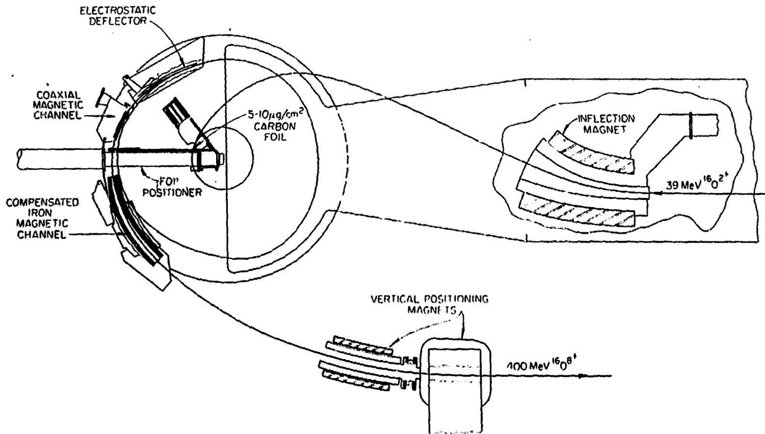
Fig. 10. The Oak Ridge cyclotron (ORIC) as modified for booster accelerator operation.
