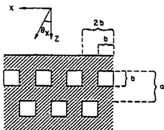
Figure 2a. Sampling geometry used for the Monte Carlo results shown below. The absorber material is iron; the sampling medium is argon gas at atmospheric pressure; the beam is parallel to the Z direction and randomly distributed in X. For this configuration the ratio of sampling volume to total volume is given by
