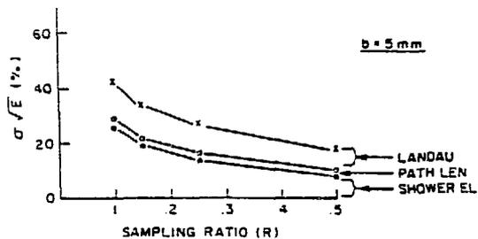
Figure 2b. Energy resolution for incident electrons, as a function sampling ratio, for  $5 \times 5 \text{ mm}^2$  sampling channels. The lowest curve corresponds to fluctuations in the number of sampled shower electrons, the next incorporates path length fluctuations, and the top curve gives the net resolution (Ref. 2).
