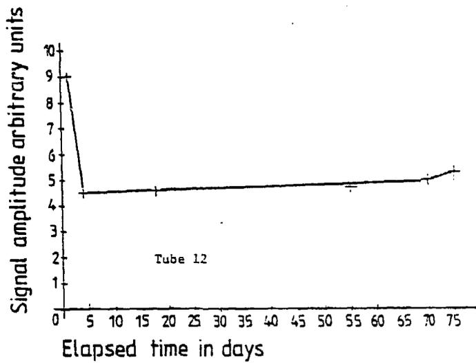
Figure 7. Time history of pulse-height measurements with two tubes in which  $\alpha$ -emitting radioactive sources have been imbedded. Due to the high ionization density produced by the  $\alpha$  particles they provide a more sensitive check on impurity effects than minimum ionizing tracks. Tube 11 was operated with an  $^{241}\text{Am}$  source with an applied voltage of 1 kV; tube 12 had a  $^{238}\text{U}$  source and was operated at 3 kV.
