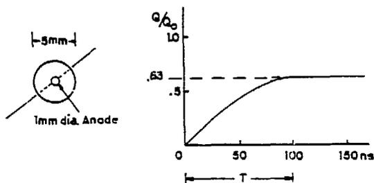
Figure 5. Time development of the signal charge for a track crossing an ion tube in the illustrated geometry, producing ionization charge  $Q_0$ . The gas mixture is 90% argon/10% methane, with the central anode at +4 kV. The time (T) for full signal collection is 100 nsec.
