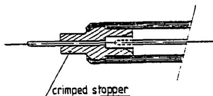
Figure 4. Construction details of the ion tube.
