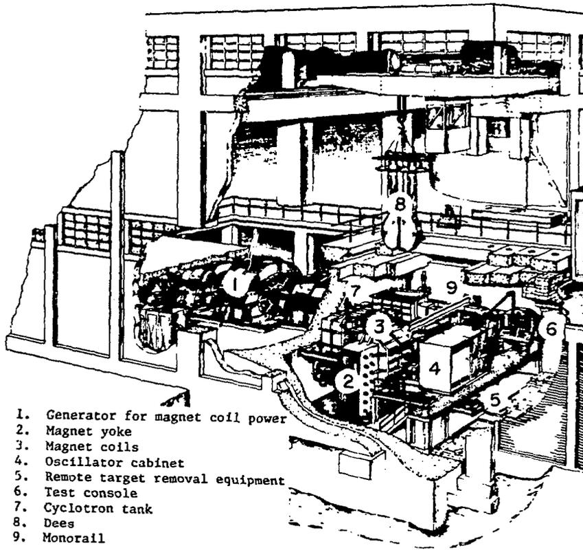
1. Generator for magnet coil power
