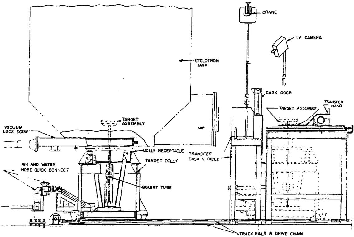
Fig. 5. Remote Equipment for Target Handling
