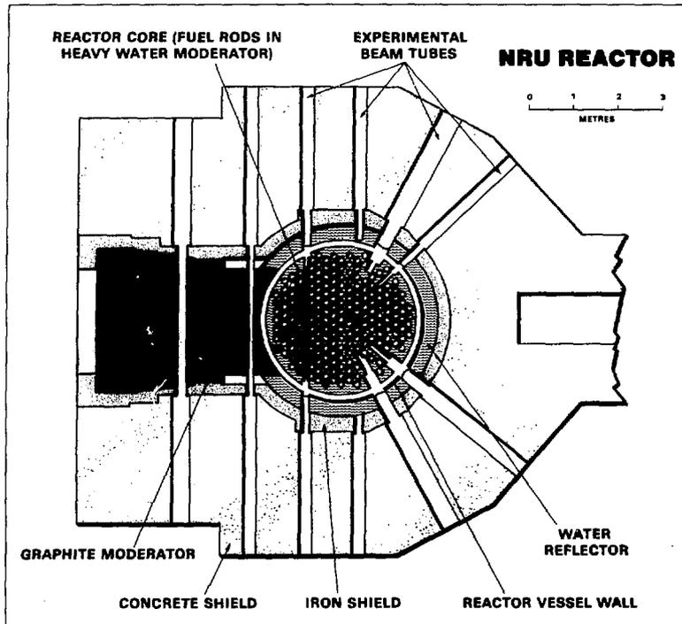
Fig. 2 Plan view of the NRU reactor showing the penetration of experimental beam tubes through the concrete and iron shields to the region of high neutron flux in or near the core. Tubes of different sizes and locations with respect to the core are provided.
