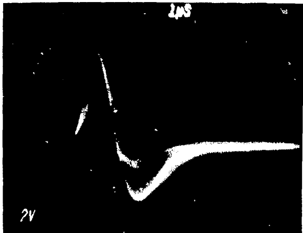
Fig. 13. Oscilloscope display of an amplifier test point signal with the ^{252}\text{Cf} calibration source in the detector. Vertical scale = 2 V/ div; horizontal scale = 1 \mu\text{s} / div.
