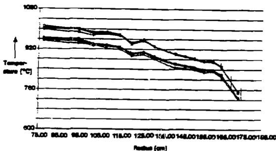
Radial Temperature Profile in the Top-Reflector of AVR
