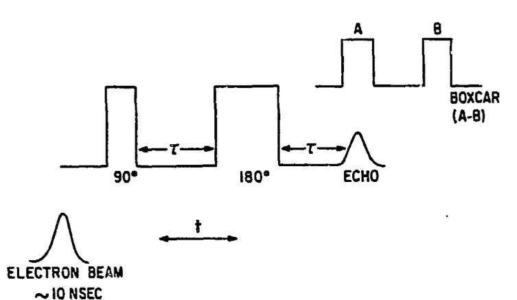
Figure 3. Timing sequence of the electron beam pulse, microwave pulses and the observation (boxcar) gates.
