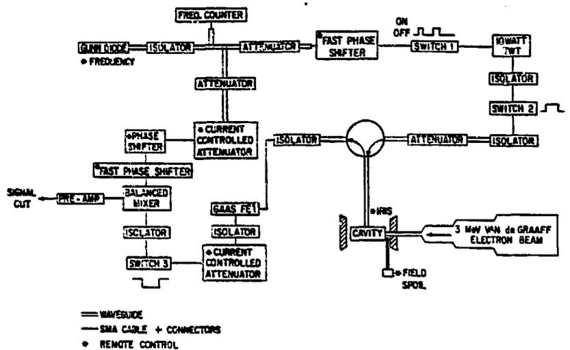
Figure 2. Schematic of microwave network used in pulsed EPR experiments with the Van de Graaff accelerator. The switching functions of the microwave switches are also indicated.
