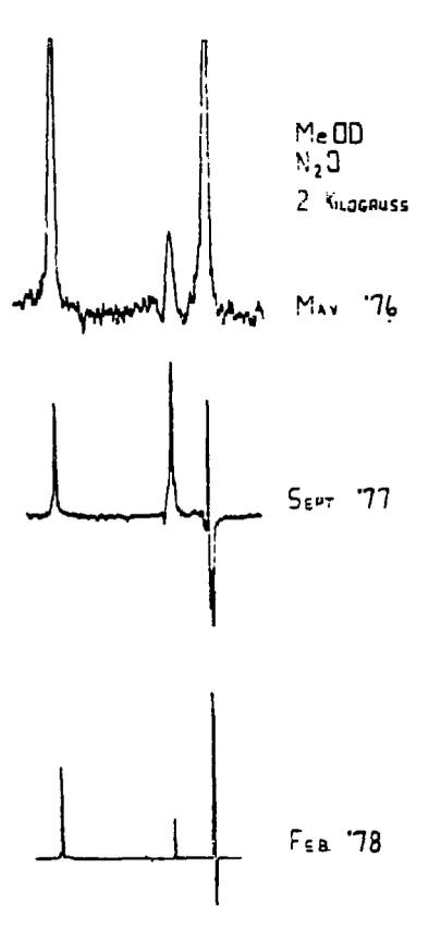
Figure 11. NMR spectra showing CIDNP of products observed in methanol radiolysis. Evolution of experimental technique is illustrated. Top and middle spectra were obtained using CW-NMR. Bottom spectrum was obtained using FTNMR.
