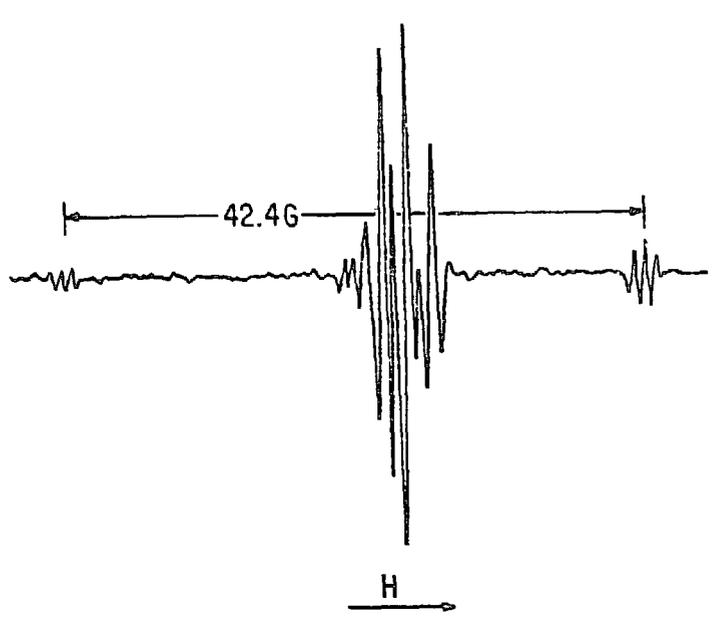
Figure 9. "FID" spectrum of the acetate radical (at 1 usec) obtained by using only a 90° pulse.
