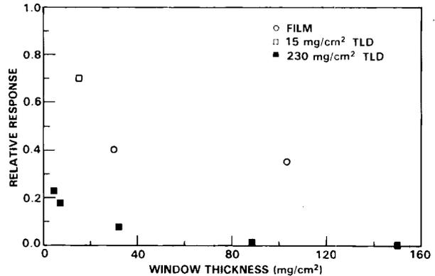
**FIGURE 3.** Low-Energy Beta Response [ $^{85}\text{Kr}/^{90}\text{Sr}-^{90}\text{Y}$ ].
