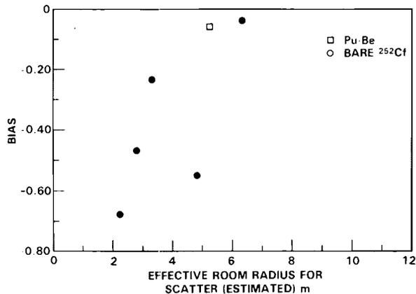
**FIGURE 4.** TLD-Albedo Dosimeter Performance as a Function of Effective Irradiation Room Radius. The effective room radii were adjusted to represent relative scatter contribution at 50 cm.
