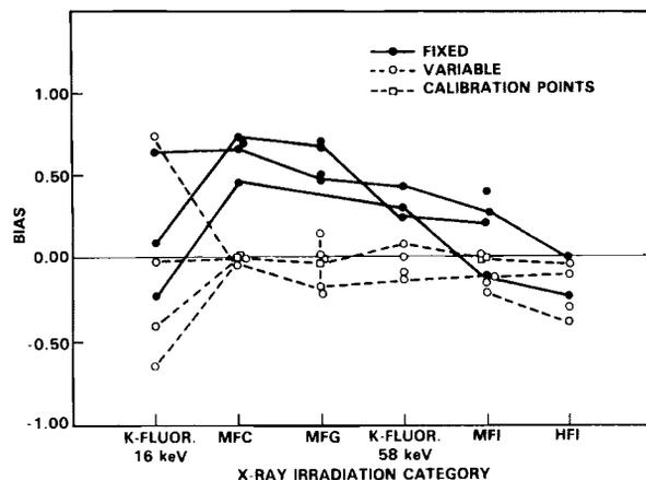
**FIGURE 1.** X-Ray Shallow-Dose Performance of TLD Dosimeters. The dosimetry systems were calibrated using PNL irradiations.
