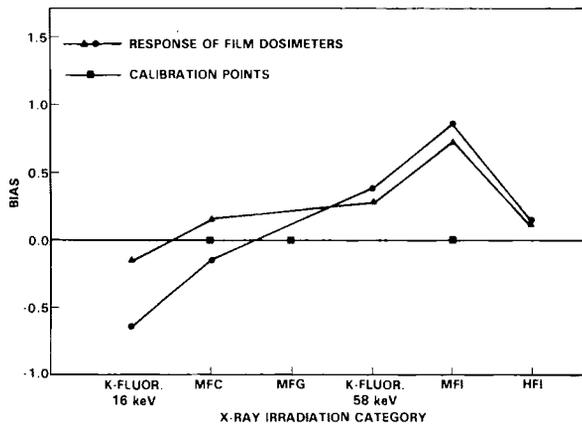
**FIGURE 2.** X-Ray Shallow-Dose Performance of Film Dosimeters. The dosimetry systems were calibrated using PNL irradiations.
